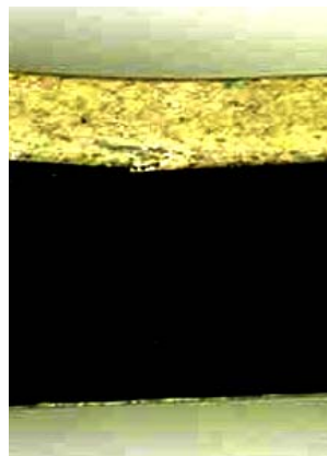
Fig.VII-4: Crack kinking out of the interface plane
