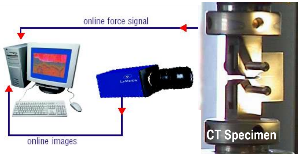
Fig.V-4: Optical Crack Tracing
