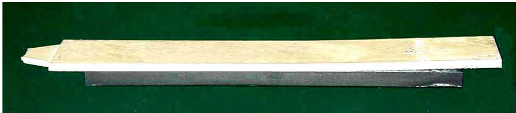
Fig.V-2: Examples of a precracked double cantilever beam specimen (thickness of resin: 4mm, thermoplastic 2mm)
