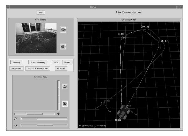
Figure 4.5: Path covered by Dala during Run 1. The trajectories labeled "rflex" and "steo" represent the position estimated respectively by odometry and visual odometry along the path. The visual odometry is indispensable even if it considerably slows down the robot.
