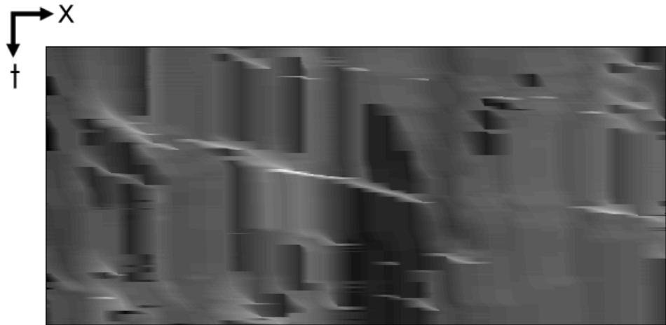
Fig. B.2: Elevation of the bed surface b_s(x, t) as a gray scale image. Image dimensions: \Delta x = 220 mm, \Delta t = 2 s. White: w_f(x, t) = +15.5 mm, black: w_f(x, t) = -7.3 mm versus the mean value. For experimental conditions, see Tab. 4.2, experiment D.
