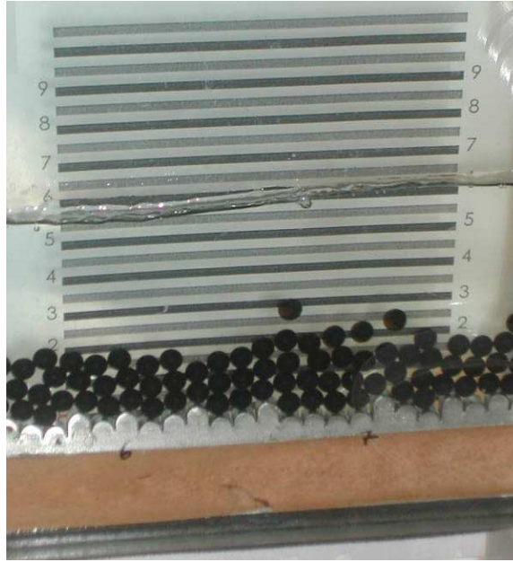
Fig. 2.5: Scales attached at the back of the channel allowed us to measure the bed and water elevation at several x -positions. Here, flow is running from right to left.
