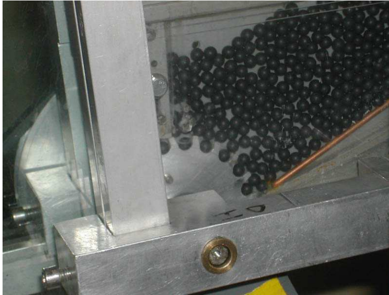
Fig. 2.4: Bead supply system of the channel (transport direction from right to left). The beads were guided by the reservoir to the transport wheel which was equipped with 20 hollows (diameter: 76 mm, width: 4.5 mm). In the background part of the pulley and the V-belt can be seen.
