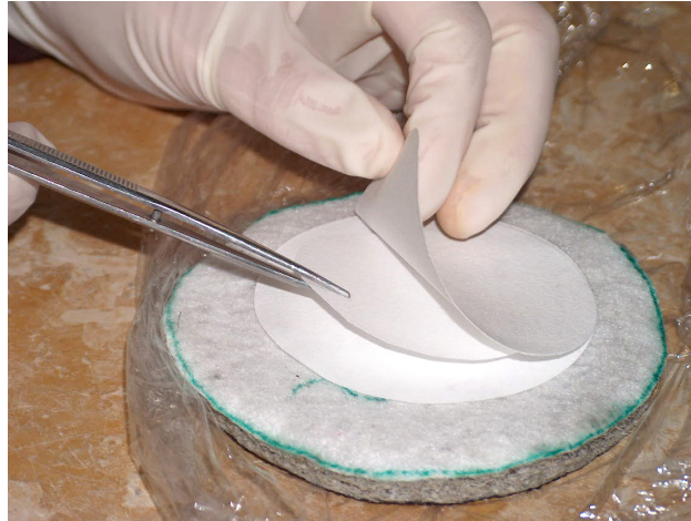
Figure 6.1 – Removing the filter paper
