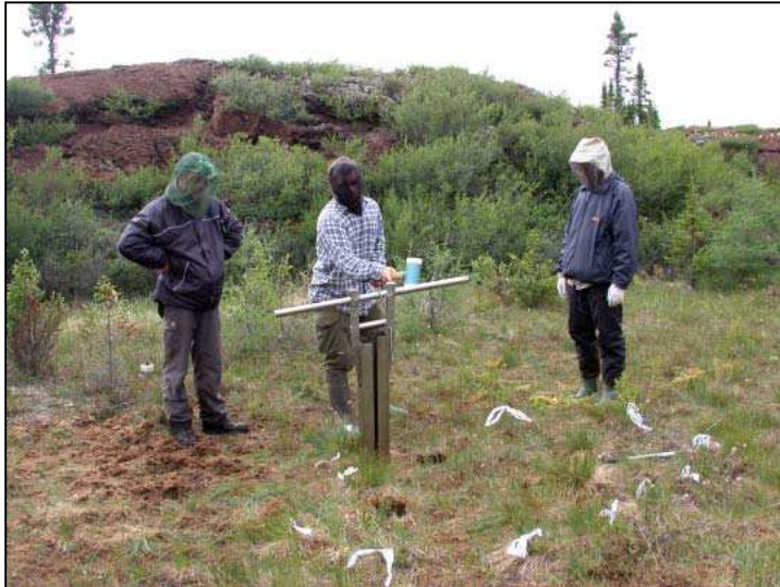
Photo 6. The Wardenaar corer is pushed down using a sledge hammer
