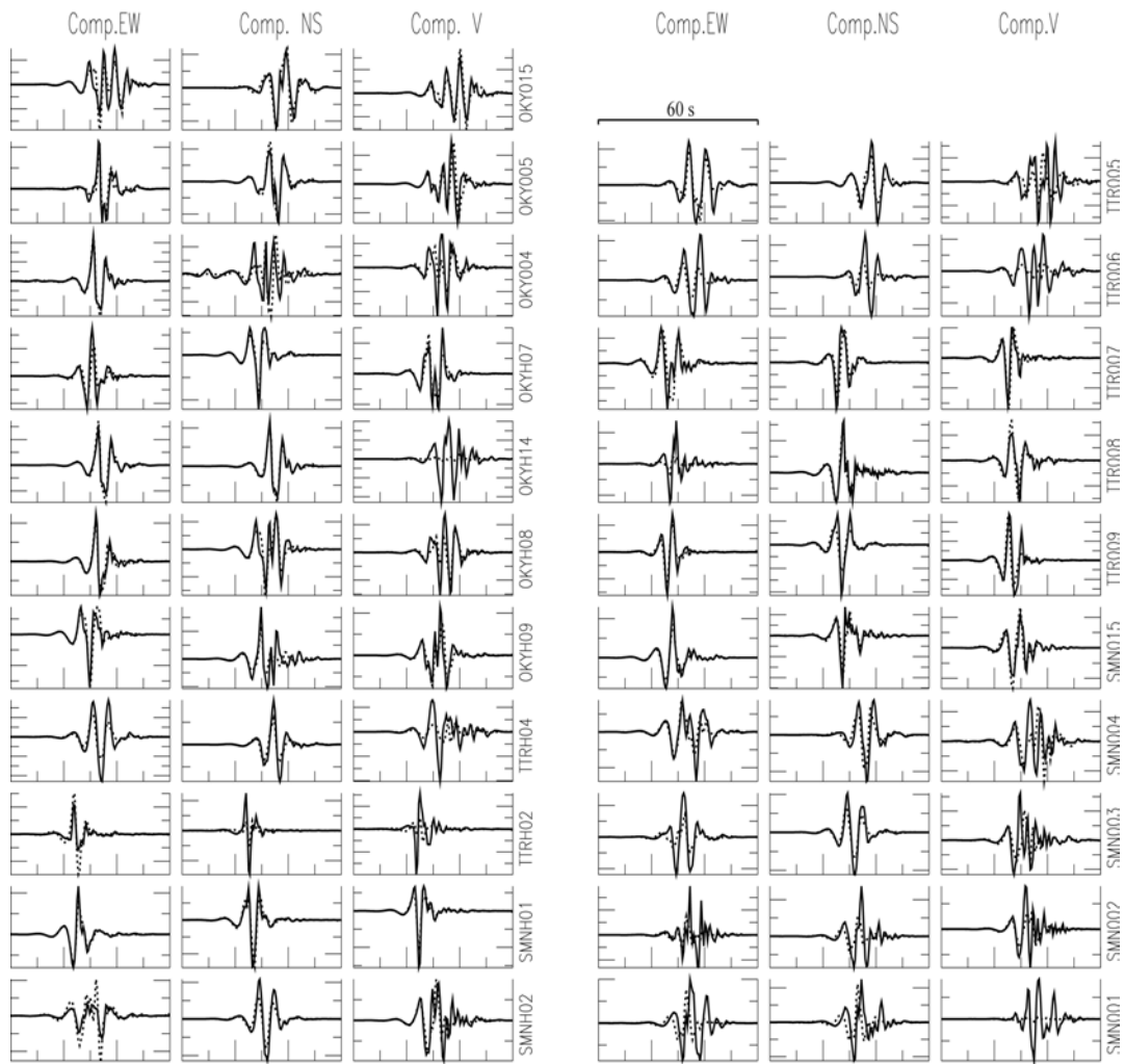
Figure 8. Observed (solid line) and synthetics (dashed line) strong motion records. Original acceleration waveforms are band-passed in the frequency range 0.1-1.0 Hz using a two-pole Butterworth filter applied forward and backward then doubly integrated to obtain the particle displacement. The vertical components of some strong ground motion are not used in the inversion (see Table 1) because of incomplete knowledge of the seismic velocity structure. All components (synthetics and observed) at each station are normalized with the data peak amplitude. Each pair of observed and calculated seismograms is plotted at the same amplitude scale.
