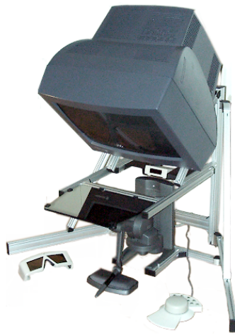
Figure 14: The haptic desktop display. The PHANTOM device, a stylus that allows interaction with 6 degrees of freedom (3 rotations and 3 translations), is positioned beneath a semi-transparent mirror. The graphics are projected through the mirror to obtain co-location of graphics and haptics.
