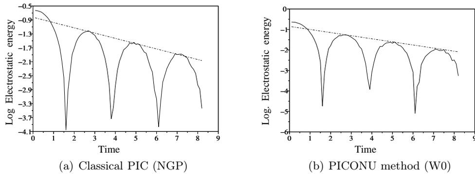
FIG. 7.3 – Landau damping with  $\alpha = 0.1, k = 0.5$ . Electrostatic energy
