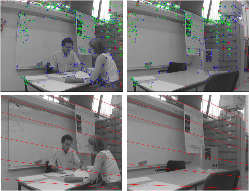
Figure 2.15: Matching with viewpoint change and moving elements in the scene. 4 wrong matches out of 204 matches are detected by evaluating with the distance computed using epipolar lines - the matching time is 140ms.
