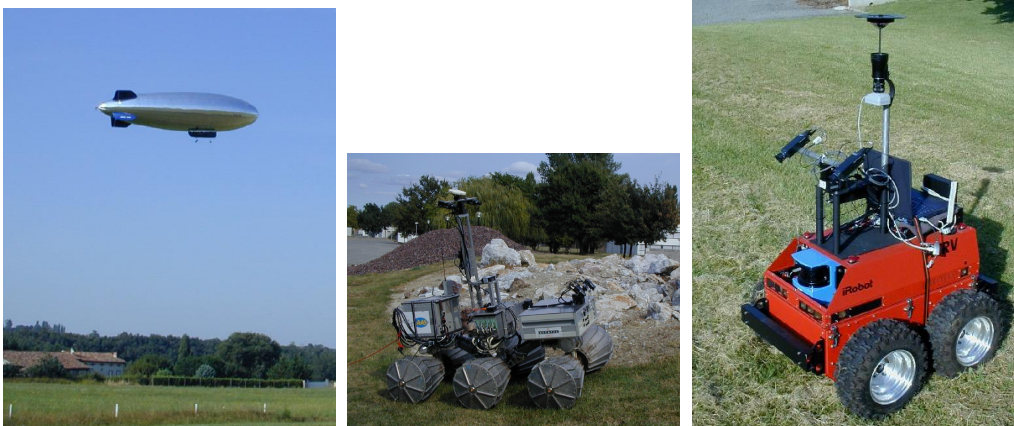
Figure 4.1: Karma, Lama and Dala: the three robots used to gather stereovision images pairs respectively from low altitudes, on a rough unstructured terrain, and indoor.
