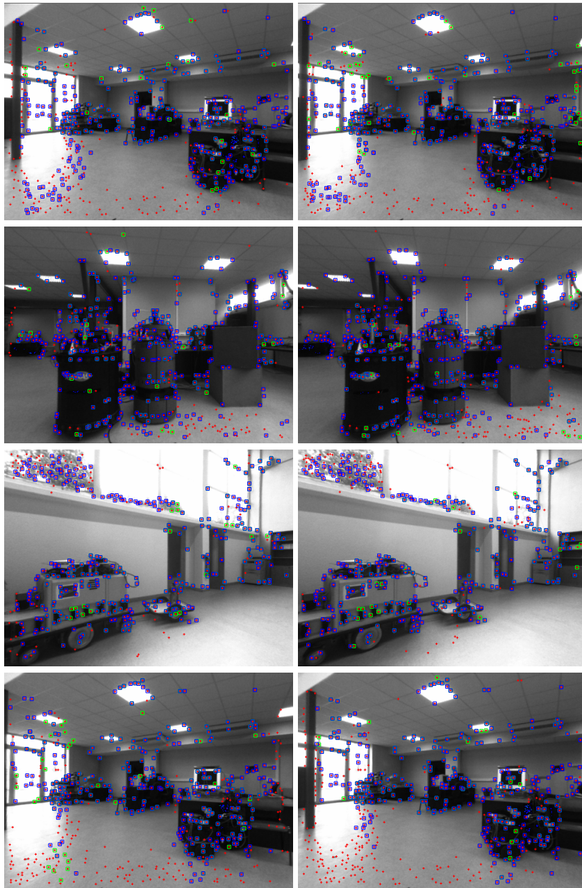
Figure 4.13: Interest points matched between some consecutive images of the sequence of the trajectory shown in figure 4.10. Each line shows two consecutive images, except the last one that shows the matches established between the image number 324 (end of the first loop) and the first image.
