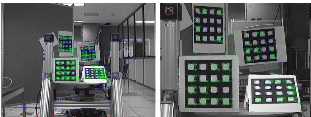
Figure 2.18: Matching with scale change: only one wrong match out of 123 matches, the matching time is 810ms.
