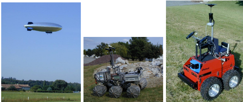
Figure 4.1: Karma, Lama and Dala: the three robots used to gather stereovision image pairs respectively from low altitudes, on a rough unstructured terrain, and indoor.
