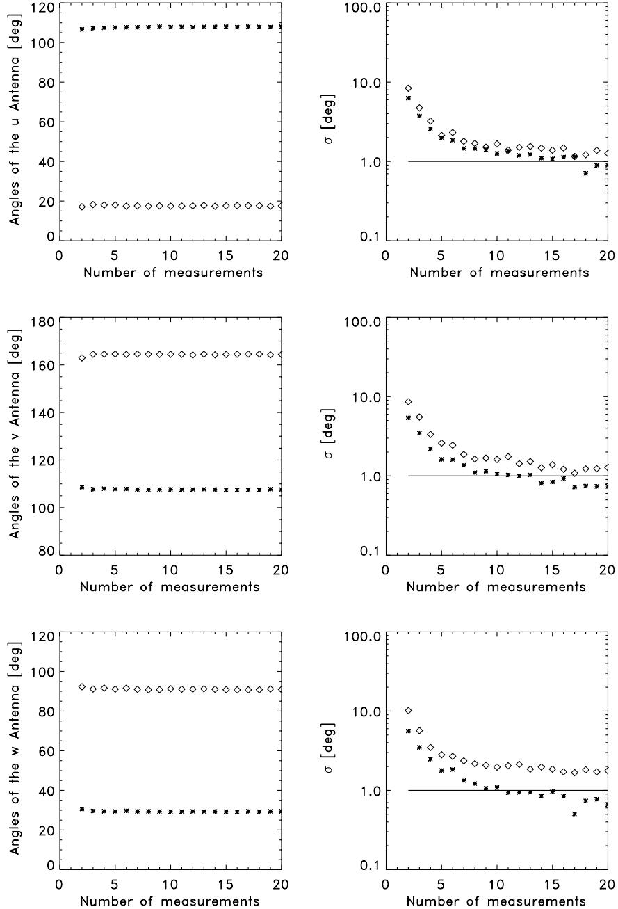
**Figure 5.** The left panels show averaged values of the colatitude (star symbol) and azimuth (diamond symbol) for the  $u$  antenna (top), the  $v$  antenna (middle), and the  $w$  antenna (bottom) versus the number of data sets to be used. The right panels give the corresponding standard deviations.
