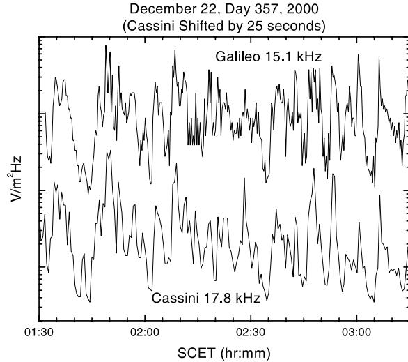
**Figure 11.** A plot of the Galileo 15.1 kHz channel (top curve) and the Cassini 17.8 kHz channel (bottom curve) for the period from 0130 to 0315 on day 357, 2000. The Cassini data has been shifted by 25 s, the difference in the light time from Jupiter to each of the spacecraft. As can be seen, both spacecraft detect QP bursts with very similar periods and structure, even though Galileo is in the magnetosphere during this event.
