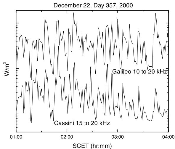
**Figure 12.** A plot of the integrated power flux from 10 to 20 kHz (1 min averages) of the QP emissions as measured by Galileo (top curve) and from 15 to 20 kHz by Cassini (bottom curve) for 22 December 2000. The Cassini data has been shifted downward to allow a more easy comparison of the data. The QP bursts observed by the two spacecraft are very similar, with much of the fine structure of the QP bursts appearing at both spacecraft.
