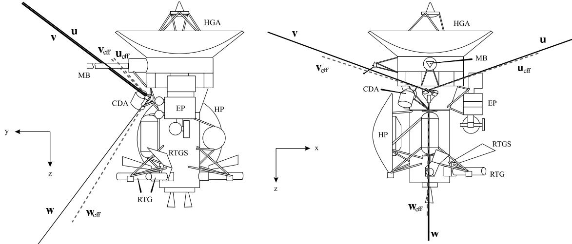
**Figure 1.** Sketch of the Cassini spacecraft adapted from Rucker *et al.* [1996]. Abbreviations are Magnetometer Boom (MB), Cosmic Dust Analyzer (CDA), Huygens Probe (HP), shades of the Radioisotope Thermoelectric Generators (RTG-S), Experimental Platform (EP), and High-Gain Antenna (HGA). The mechanical antenna elements are drawn as solid lines, and the corresponding effective antenna axes derived in this paper are shown as dashed lines.
