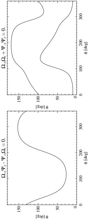
FIGURE 4: Left : the curve is the locus of the points for which  $\Omega_{+X}\Psi_Z - \Psi_{+X}\Omega_Z = 0$ . Right : the 2 curves are the locus of the points for which  $\Omega_{+X}\Omega_Z + \Psi_{+X}\Psi_Z = 0$ . The  $\theta$  and  $\phi$  coordinates are the colatitude and azimuth in the spacecraft frame. Those curves correspond to undetermined configurations in the general case DF analytical inversion.
