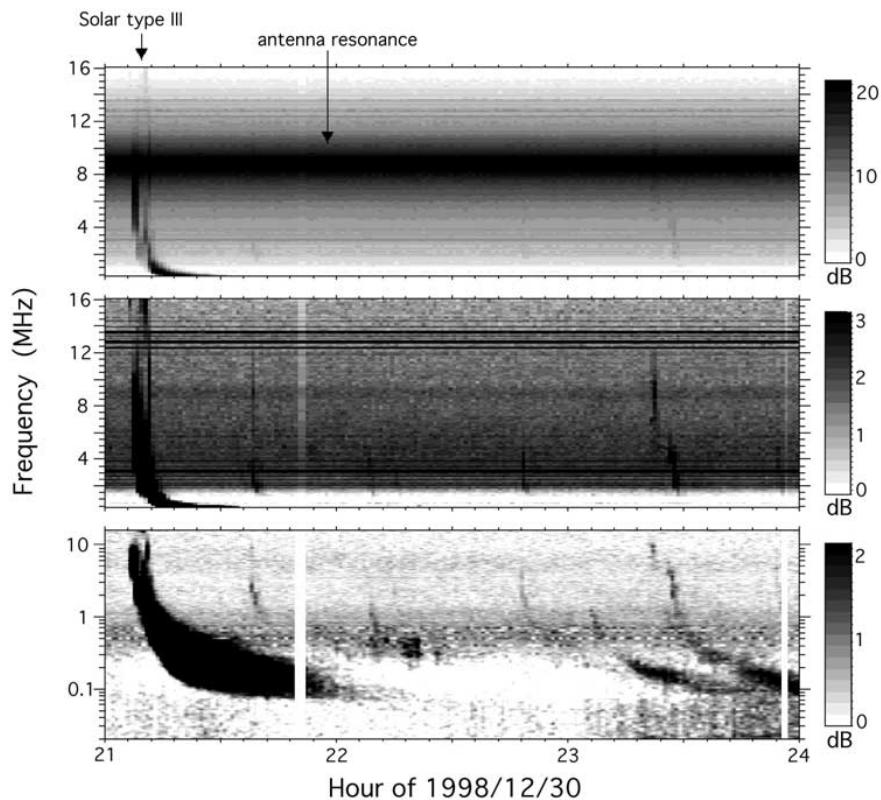
**Figure 3a.** Quiet interval of HFR data recorded with the dipole antenna (channel 1). Top panel displays raw data with linear frequency scale. Middle panel displays the dynamic spectrum after subtraction of a frequency-dependent background. Bottom panel shows the whole HFR band after background subtraction, with log frequency scale. One intense and several weak solar type III bursts are detected.
