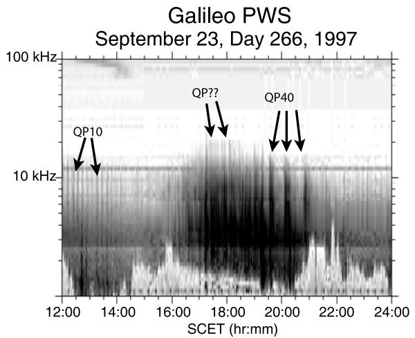
**Figure 2.** Frequency-time spectrograms showing typical QP bursts detected by Galileo in the Jovian magnetosphere. The QP bursts appear as enhancements of the trapped continuum and often display a wide range of periods, ranging from 1 or 2 min to 60+ min. In this example,  $\sim 10$  min,  $\sim 40$  min, and somewhat random periods are observed.
