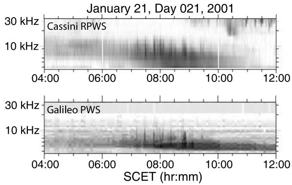
**Figure 7.** Frequency-time spectrograms showing QP bursts detected by Cassini (top panel) and Galileo (bottom panel) from 21 January 2001, when both spacecraft are in the solar wind. QP bursts are detected by both spacecraft from about 0700 to 1000 SCET. The QP bursts detected by both spacecraft range in frequency from about 5 kHz to 15 kHz. Cassini is located about  $320 R_J$  from Jupiter and at 20.5 hours LT, while Galileo was about  $144 R_J$  from Jupiter and at 16.9 hours LT.
