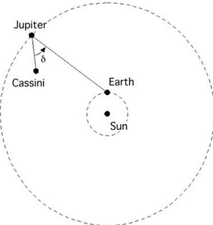
**Figure 12.** Cassini-Jupiter-Earth geometry at the time of the observations of Figure 11. Distance from Cassini to Jupiter was 0.21 AU, while distance from Earth to Jupiter was 4.2 AU, hence a light travel time delay of 33.2 min. Cassini-Jupiter-Earth angle was  $\delta \sim 13.4^\circ$ , corresponding to a delay of 22.1 min between illumination of Cassini and Earth by a beam rotating with Jupiter (93 min for a beam rotating with Io).
