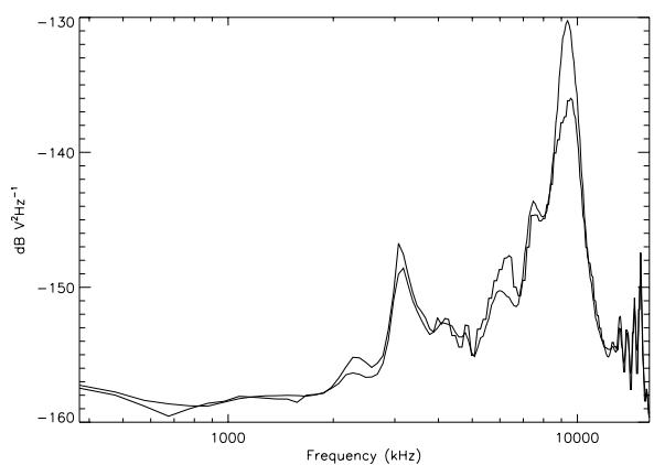
**Figure A1.** Background noise spectrum (including galactic plus receiver noise) measured by the RPWS-HFR with the monopole antennas during “quiet” intervals of a few hours far from Jupiter (lightface line). The boldface line was computed as the lower 5% occurrence level detected at each frequency during a 6 month interval centered on the Jupiter flyby. It serves as our reference for the background spectrum ( $Pg + Pr(f)$ ) for Jupiter studies. For more details, see Appendix A.
