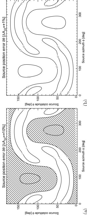
FIGURE 11: Error on source position  $\delta\theta$  in case of a 10% (a) and 1% (b) increase of the flux intensity  $S$  between the 2 successive 2-antenna data-sets in DF mode. The region for which  $\delta\theta > 2^\circ$  has been hatched. The  $\delta\theta$  errors are proportional to the flux variation. Lines are iso-contours in degree.
