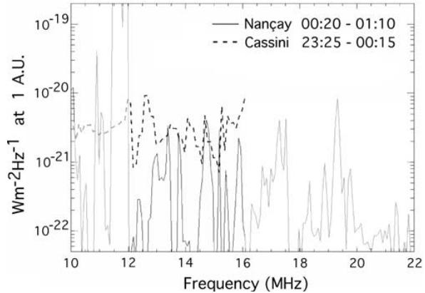
**Figure 13b.** Comparison of the spectra measured in Nançay between 0020 and 0110 and by Cassini 55.3 min earlier (time intervals arrowed in Figure 11). The common spectral range is emphasized. A broad intense interference pollutes Nançay data between  $\sim 11.5$  and 12 MHz.
