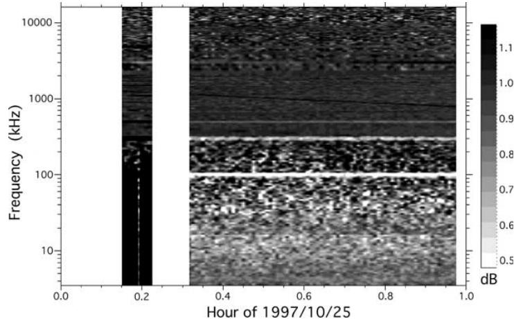
**Figure 2a.** Dynamic spectrum of the receiver's output in HFR channel 1 before deployment of the dipole antenna. Background noise fluctuations and weak interference lines are detected.
