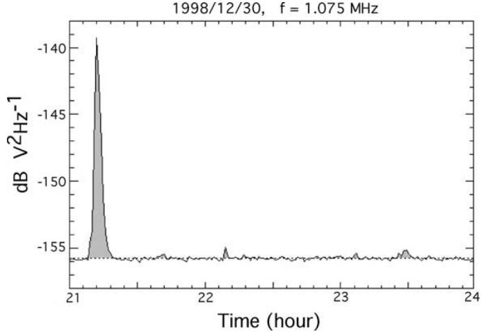
**Figure 3b.** Cut of Figure 3a at frequency  $f \sim 1$  MHz. Time resolution is 60 s per sample. Type III emission is gray shaded. The background level is indicated by the dotted line. Its fluctuations are less than  $\pm 0.2$  dB.
