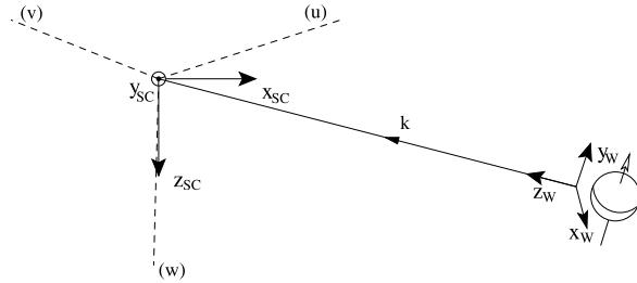
**Figure E1.** Wave frame ( $\mathbf{x}_w, \mathbf{y}_w, \mathbf{z}_w$ ) and spacecraft frame ( $\mathbf{x}_{SC}, \mathbf{y}_{SC}, \mathbf{z}_{SC}$ ). The antenna directions are shown in dashed lines. Quantity  $\mathbf{z}_w$  is colinear to the wave vector  $\mathbf{k}$  and the  $\mathbf{y}_w$  is in the plane containing  $\mathbf{k}$  and the rotational axis of the observed planet.
