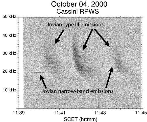
**Figure 1.** An example of a series of Jovian type III radio bursts (also known as quasi-periodic (QP) bursts) detected by the wideband receiver on Cassini on 4 October 2000, at a distance of  $1140 R_J$ .
