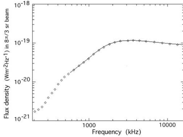
**Figure 1.** Galactic low-frequency model radio spectrum  $S_g(f)$  derived from *Dulk et al.* [2001] (continuous line) and *Manning and Dulk* [2001] (diamonds). Their combination is our reference galactic background flux density spectrum.
