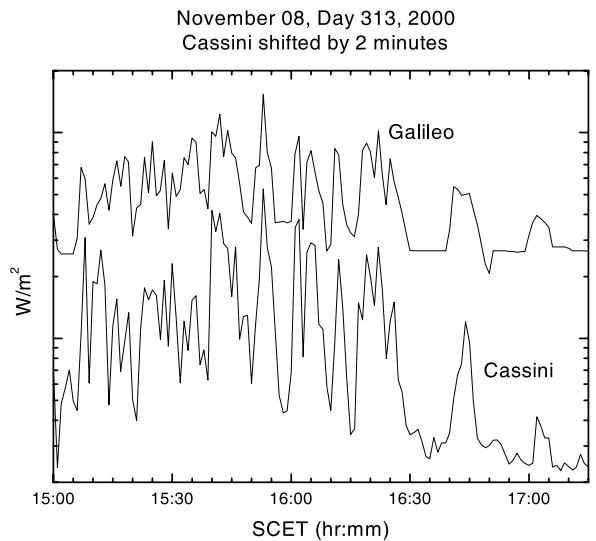
**Figure 5.** A plot of the integrated power flux from 15 to 20 kHz (1 min averages) of the QP emissions as measured by Galileo (top curve) and Cassini (bottom curve). The Cassini data has been shifted downward to allow a more easy comparison of the data and “earlier” (to the left) by 2 min to account for the difference in the light time from Jupiter to each of the spacecraft (actual difference is 109 s, or 1.82 min). As can be seen, the QP bursts observed by the two spacecraft are very similar.
