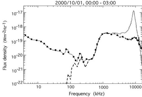
**Figure 5a.** Average spectrum of Jovian radio emissions detected on 2000/10/01, 0000 to 0300 with the HFR dipole antenna. Distance to Jupiter is  $1184 R_J$  or 0.565 AU. Spectra obtained through short dipole calibration (continuous line) and calibration based on the galactic background (dashed line) are compared (see text). Final (composite) calibrated spectrum is indicated by solid dots.
