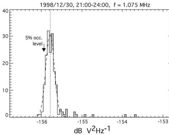
**Figure 3c.** Histogram of intensities in 60 s samples of Figure 3b, at  $f = 1.075$  MHz. The gaussian distribution (dashed) corresponds to the galactic noise plus receiver noise and their fluctuations at this frequency. The average value of  $(P_g + P_r)$  at 1.075 MHz corresponds well to the mode of the histogram (dotted line). The higher intensity tail (gray shaded) corresponds to measurements of the type III emission. The limit of the lower 5% occurrence level is arrowed.
