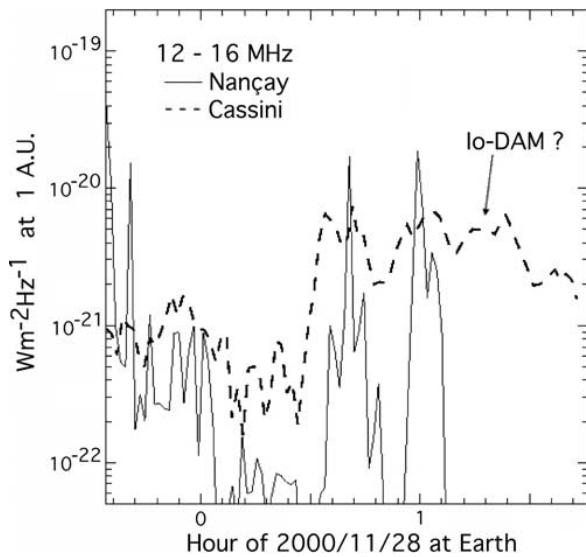
**Figure 13a.** Time variations of the flux density measured by Cassini and in Nançay, averaged over the range 12–16 MHz (arrowed in Figure 11). In the case of Nançay data, only those channels not dominated by interference were taken into account within that band. Time is UT at Earth: Cassini spacecraft event time has been shifted by +55.3 min.
