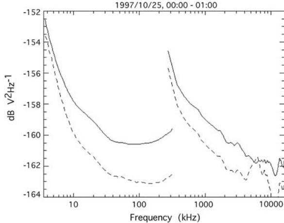
**Figure 2b.** Minimum noise levels measured before antenna deployment at the inputs of channel 1 (dipole D shown by continuous lines) and channel 2 (monopole Z shown by dashed lines) in the two HFR subbands (3.5–320 kHz and ~300–16100 kHz).
