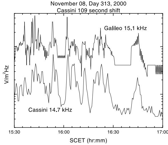
**Figure 6.** A plot of the Galileo 15.1 kHz channel (top curve) and the Cassini 14.7 kHz channel (bottom curve) for the period from 1530 to 1700 on day 313, 2000. As can be seen, both spacecraft detect the QP emissions with very similar periods and structure. The Cassini data has been shifted downward to more easily compare the two curves and “earlier” by 109 s, which is the difference in the light time from Jupiter to each of the spacecraft.
