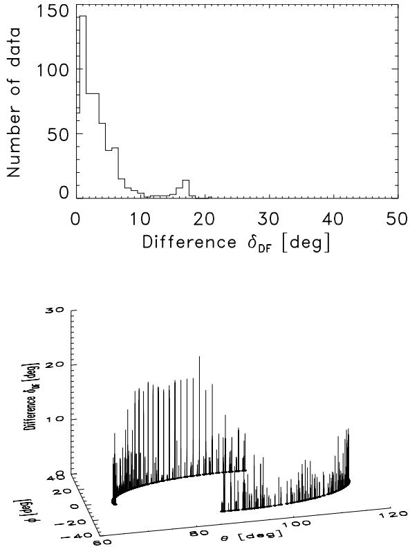
**Figure 4.** Difference (solid lines) between the DF retrieved values and Jupiter's position. The top panel shows the error occurrences as a function of the error magnitude. The bottom panel gives these errors as a function of the source position (ephemeris data).
