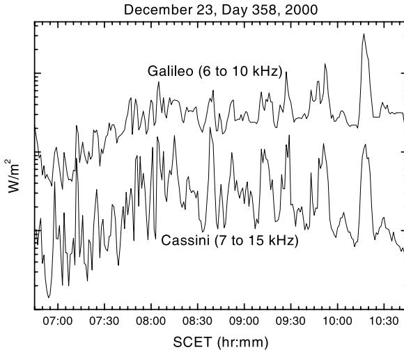
**Figure 14.** A plot of the integrated power flux from 6 to 10 kHz (1 min averages) of the QP emissions as measured by Galileo (top curve) and from 7 to 15 kHz by Cassini (bottom curve) for 23 December 2000. The Cassini data has been shifted downward to allow a more easy comparison of the data. The QP bursts observed by the two spacecraft are very similar, with much of the fine structure of the QP bursts appearing at both spacecraft.
