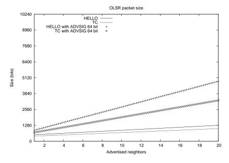
Figure 9.4: Diagram of ADVSIG overhead using 64-bit signatures.
