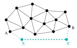
Figure 3.5: A longer wormhole created by two colluding nodes X and X'.
