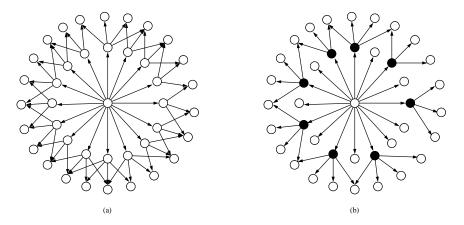
Figure 1.8: Pure fboding and MPR fboding.
