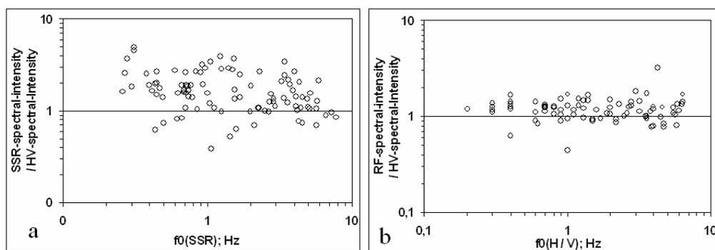
Figure 4.9 Variations of different spectral intensity ratios as a function of fundamental frequencies obtained by SSR method. The spectral intensity were calculated for the frequency  $<10$  Hz and only for the frequency range with S/N ratio  $>3$ .
