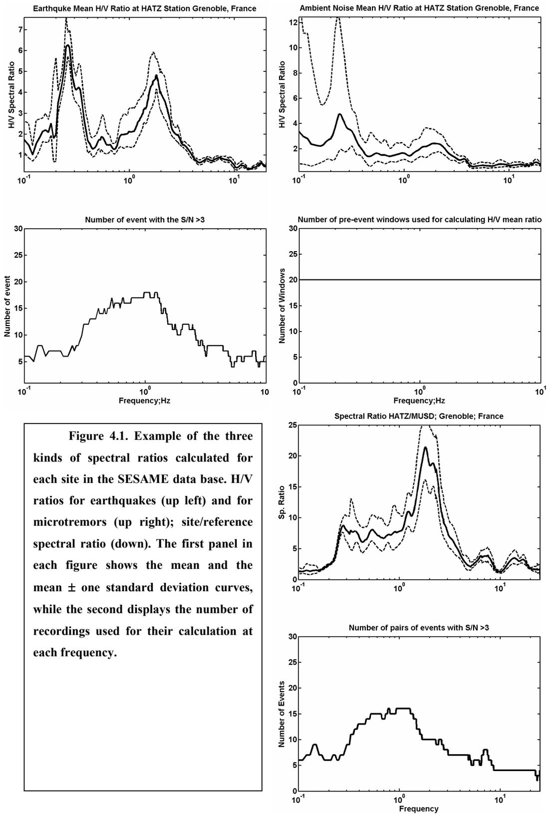
Figure 4.1. Example of the three kinds of spectral ratios calculated for each site in the SESAME data base. H/V ratios for earthquakes (up left) and for microtremors (up right); site/reference spectral ratio (down). The first panel in each figure shows the mean and the mean  $\pm$  one standard deviation curves, while the second displays the number of recordings used for their calculation at each frequency.
