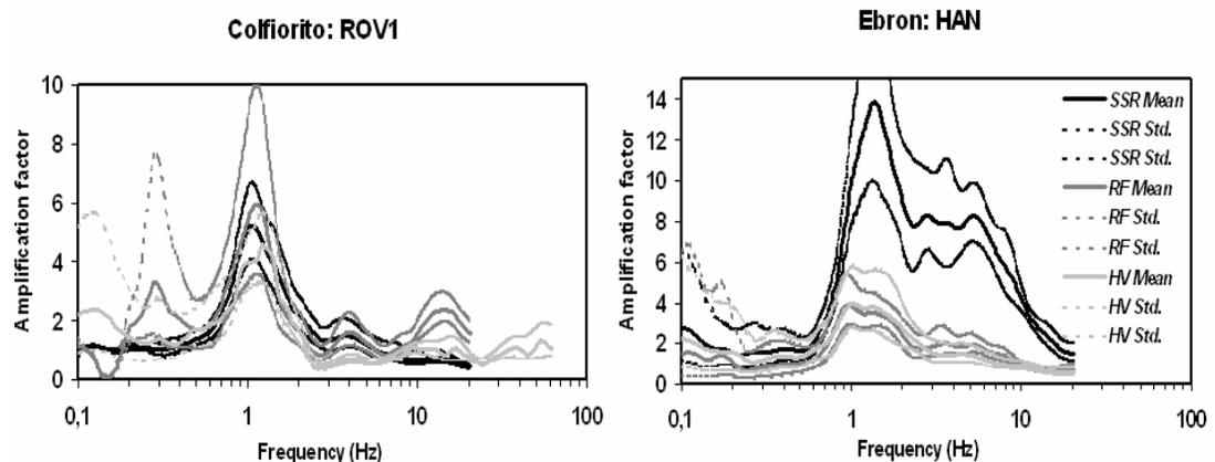
**Figure 4.2.** Two example comparison of spectral ratios obtained by the three methods: site/reference spectral ratio (SSR, black); H/V spectral ratio of earthquakes (RF, dark gray) and H/V spectral ratio of ambient vibration (HV, light gray). For each method, are displayed both the average curve, and the average  $\pm$  one standard deviation curves, These example corresponds respectively from left to right to the "Rov1" site in Colfiorito (Italy) and Han site in Ebron (France).
