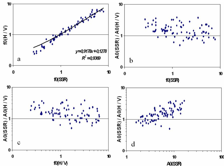
Figure 4.8 Variation of amplitude ratio  $[A_{0SSR} / A_{0HV}]$  as a function of fundamental frequencies  $f_{0SSR}$  (b) and  $f_{0HV}$  (c), and with amplification at fundamental frequency (d). These comparisons are performed on for sets exhibiting a good frequency agreement (panel "a").
