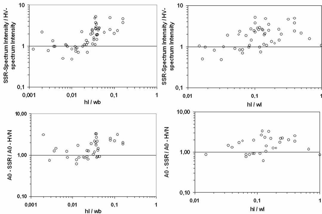
**Figure 4.12** Variation of spectral intensity ratio between SSR and H/V method with the depth/width ratio of the alluvial basin. The depth and width parameters are defined in Figure 11. The analysis is based on 30 % of the sites studied in the SESAME project for which the depth and width information were available.
