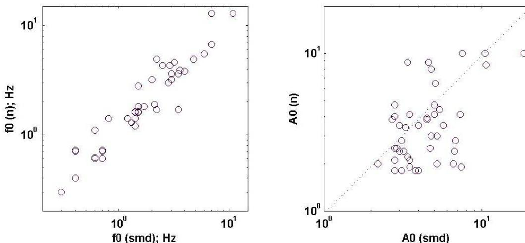
**Figure 4.10** Correlation between results from ambient noise and strong motion data for the Greek strong motion network. (left) correlation of fundamental frequencies  $f_{0n}$  with  $f_{0smd}$  ; (right) correlation of the corresponding amplitudes  $A_{0n}$  and  $A_{0smd}$ .
