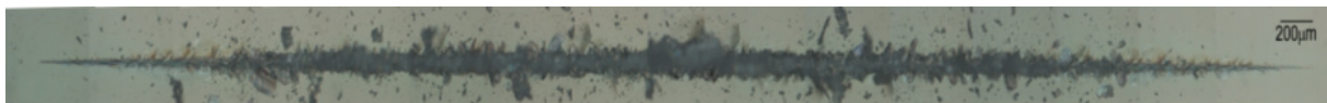
Fig. 77: Loading-unloading scratching sequence (3 N max) on an annealed standard float glass with a Vickers indenter.
