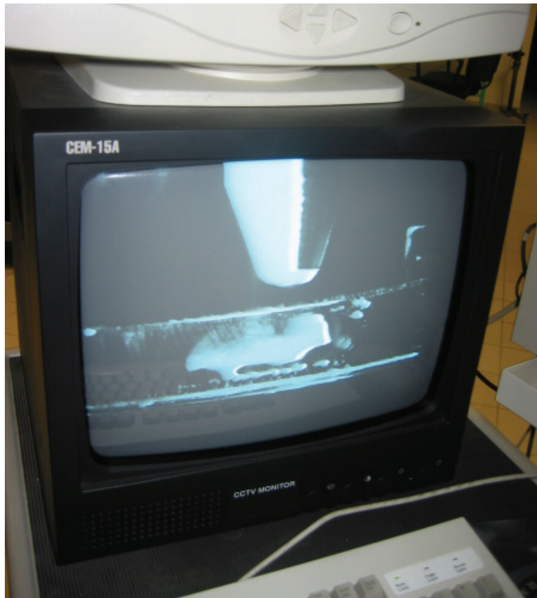
Fig. 112: Monitoring of the indenter/sample for accurate approach with the elastic double-cantilever driven by the coarse translation screw.
