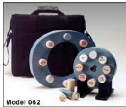
Figure IV - 25: Phantom Model 062 from CIRS compagny.
