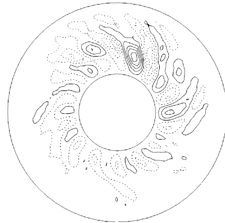
FIG. 3. Isovalues of \psi for E=10^{-5} , Ra=2 \times Ra_c , Pr=1 , with no-slip boundary conditions. This graph corresponds to chaotic oscillations, the azimuthal periodicity of the pattern is no longer preserved. Patterns of convection are localized by the shearing action of the zonal flow.
