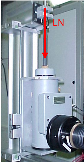
Figure 4-10: Photo of the LN/CCD camera from Princeton mounted on its stage. The yellow nut is placed on the inlet for the liquid nitrogen (LN).
