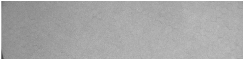
Figure 4-17: Flat field image with the PROXITRONIC image intensifier. The design of the optical coupling allows the image to illuminate the whole CCD.
