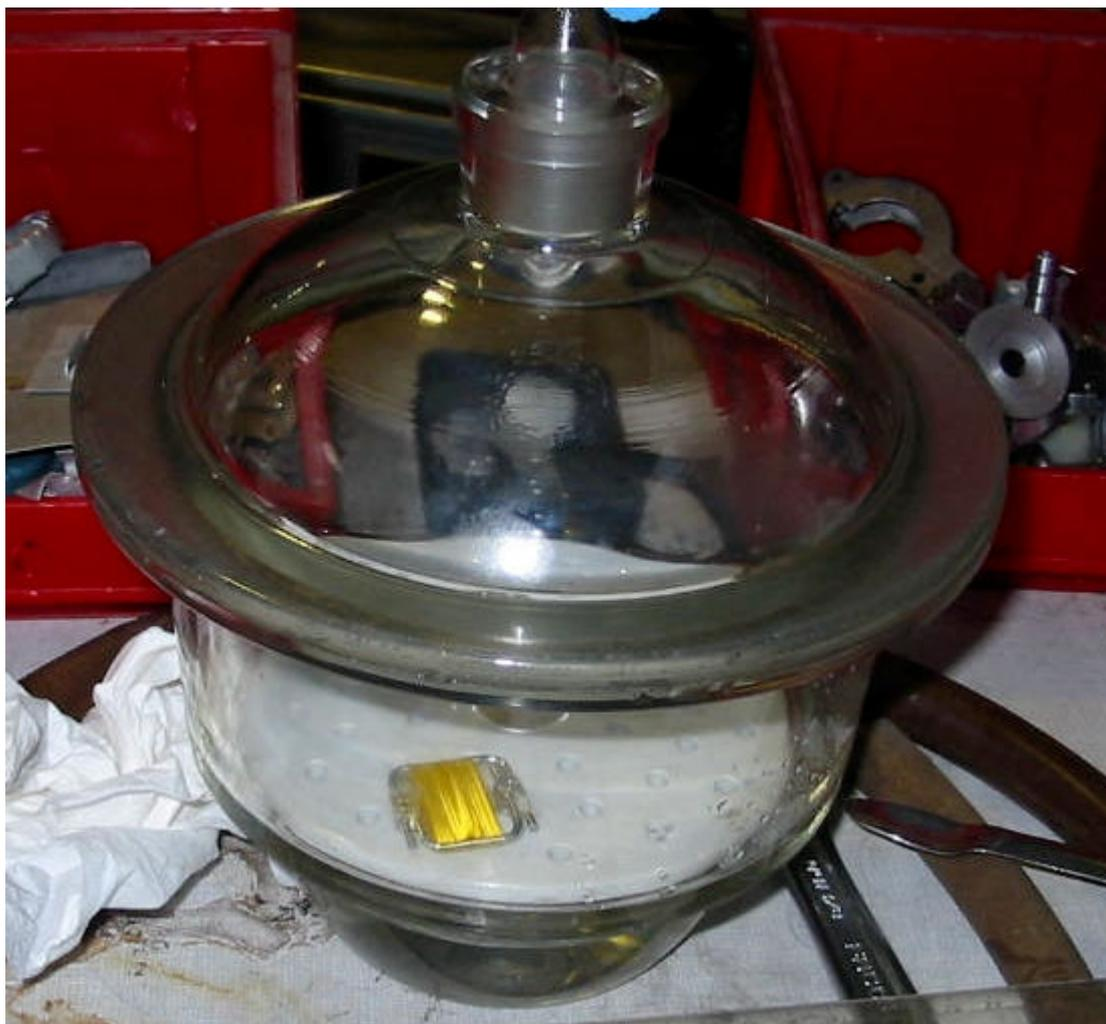
Figure 15 Hydration of the 150 mg silk sample stored in a dessicator. Water ( $\text{H}_2\text{O}$  or  $\text{D}_2\text{O}$ ) is put in the reservoir under the sample.
