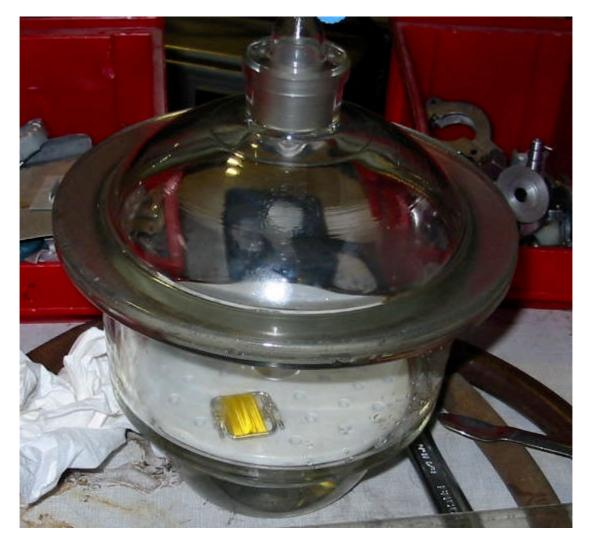
Figure 15 Hydration of the 150 mg silk sample stored in a dessicator. Water ( $H_2O$  or  $D_2O$ ) is put in the reservoir under the sample.
