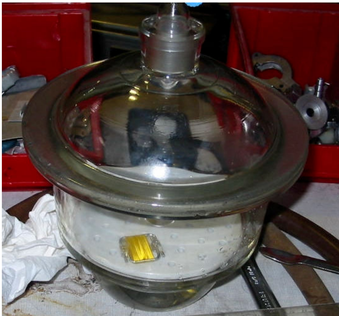
Figure 15 Hydration of the 150 mg silk sample stored in a dessicator. Water ( \text{H}_2\text{O} or \text{D}_2\text{O} ) is put in the reservoir under the sample.
