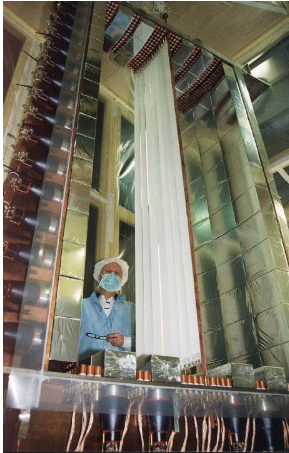
FIG. 3.14 – View of the third sector in the source mounting room just after the installation of the tellurium source.
