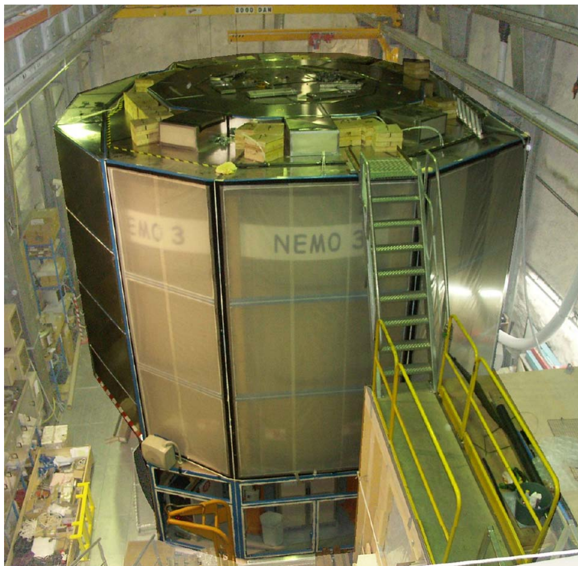
FIG. 3.144 – Picture of the airtight tent surrounding the NEMO 3 detector after its final installation in the LSM. As shown in this picture, the lower part of the tent which surrounded the electronics is now removed.
