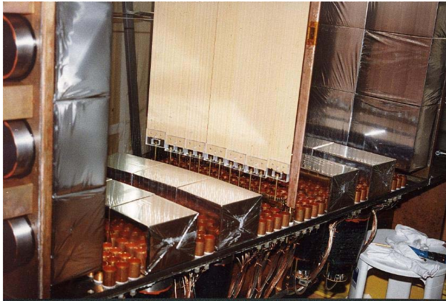
FIG. 3.77 – View of the calibration tube of one sector with the kapton window in bottom position ( z = -90 cm).
