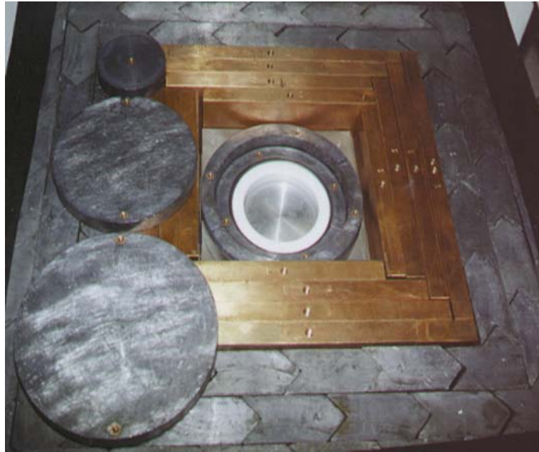
FIG. 3.92 – Picture showing a top view of Iris 400 cm 3 HPGe detector in LSM. The cryostat end-cap has a diameter of 11 cm.
