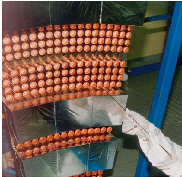
FIG. 3.52 – Photography of a petal sector during wiring. The operator passed the needle attached to stainless steel wire through the corresponding hole in the petal.
