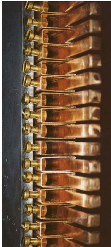
FIG. 3.83 – Detail of the copper rings used to realize the magnetic coil.
