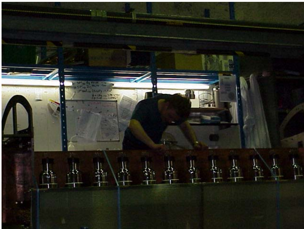
FIG. 3.90 – One sector in the LSM during the internal wall PMT attachment.
