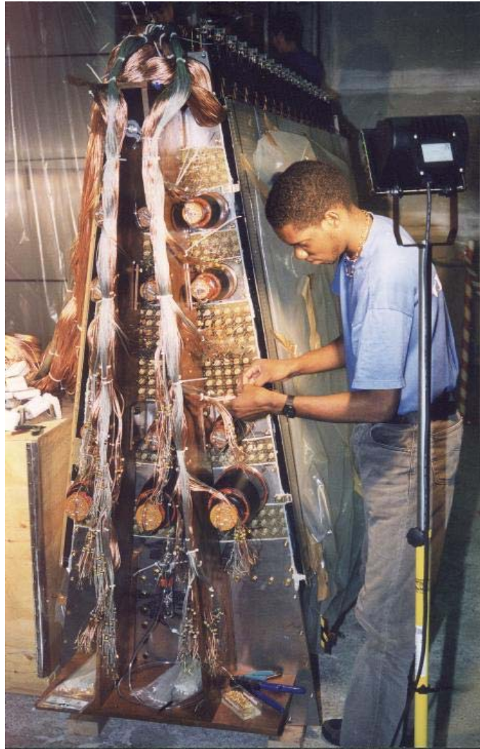
FIG. 3.56 – Picture of the anode and cathode cabling in LAL.
