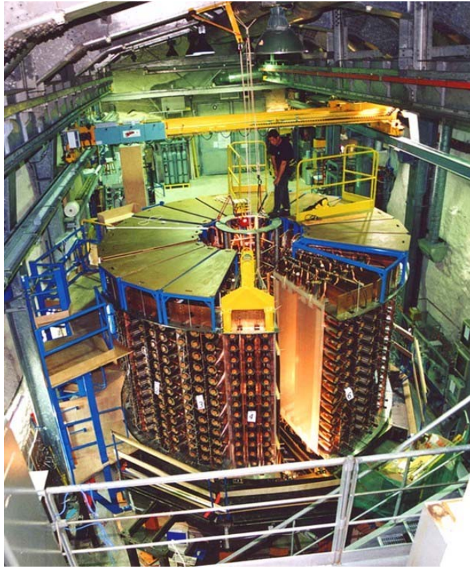
FIG. 3.12 – View of the NEMO 3 detector in the LSM before the installation of the last sector.
