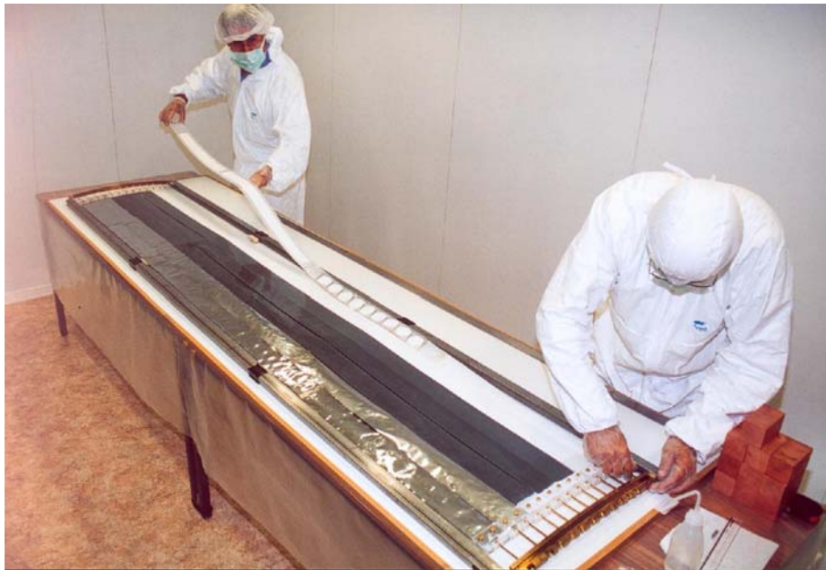
FIG. 3.31 – View of source foil production for sector 05, by attachment of the seven strips in the LSM clean room (see the calcium portion' strip with the nine 40 mm diameter disks).
