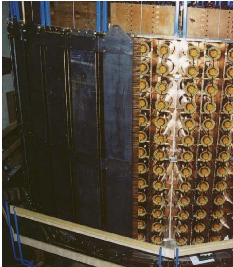
FIG. 3.84 – Picture of the coil during its installation round about the detector.
