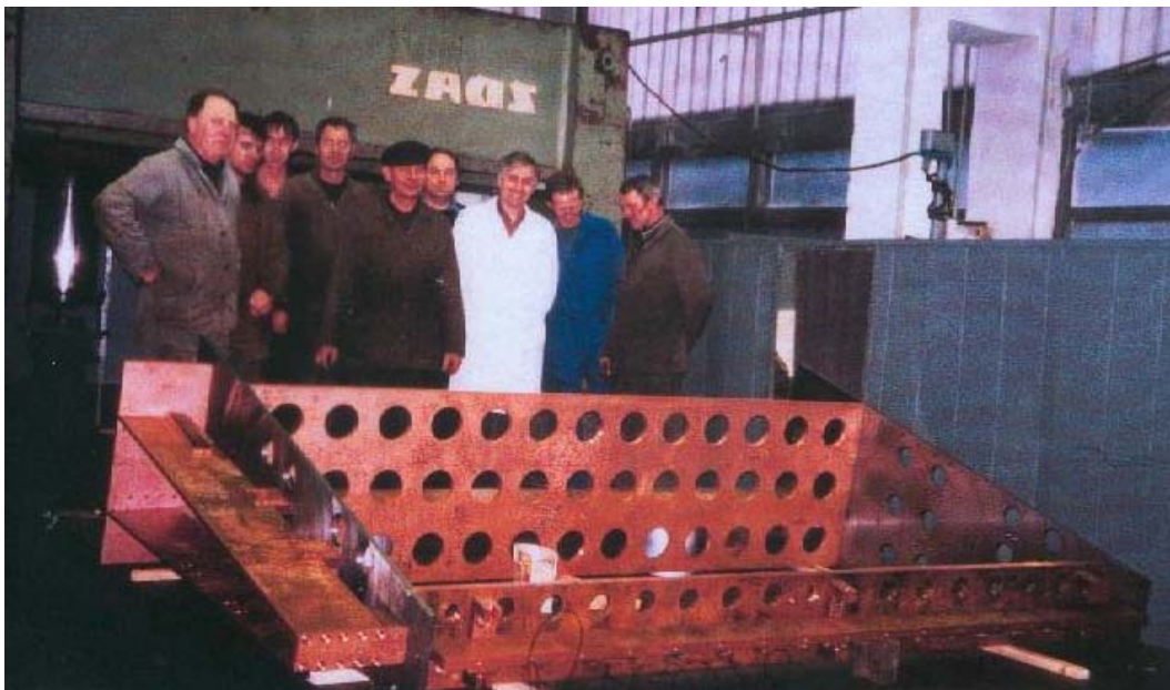
FIG. 3.20 – Test of the assembly as a sector of the first walls and petals realized at JINR Dubna.
