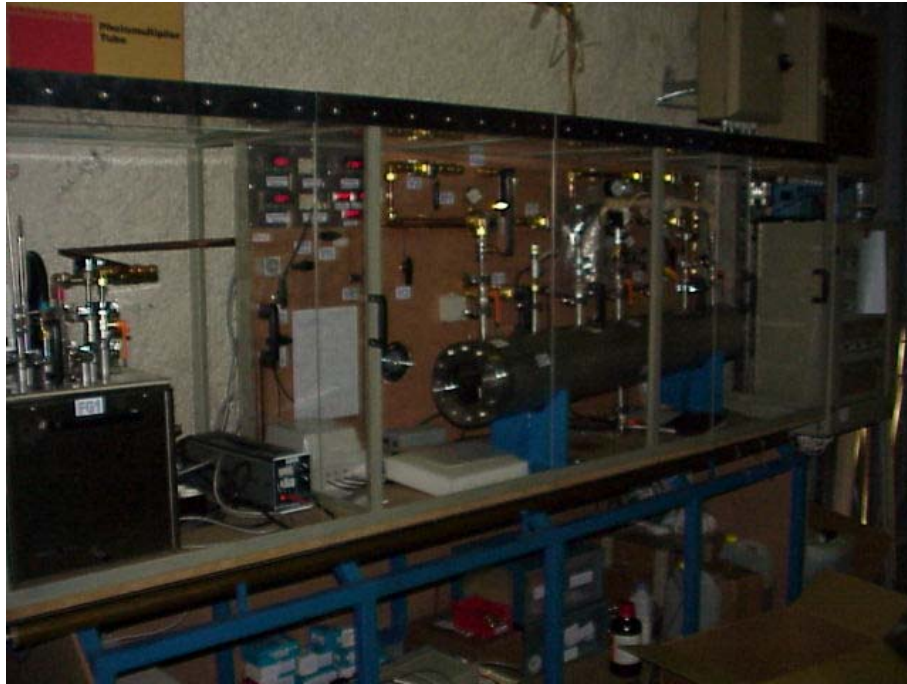
FIG. 3.87 – Picture of the gas regulation system for NEMO 3.
