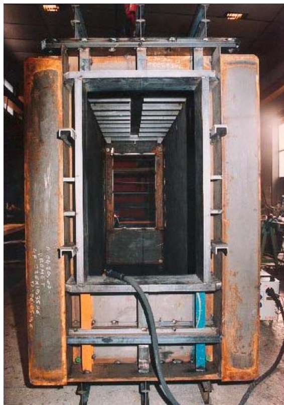
FIG. 3.53 – Realization of the special container used to test each sector after wiring.
