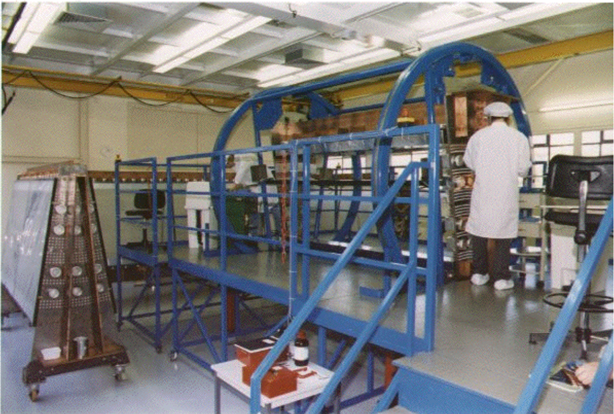
FIG. 3.50 – Photography of the gimble used for the wiring, installed in the clean room. The gimble was composed of two half-arches for an easy introduction of the sector. It used an electrical system for the 360^\circ rotation and was surrounded by many removable platforms. One can see a sector in the gimble during wiring and on the left side another sector with its protection shields, waiting for bad wire replacement after the test procedure.
