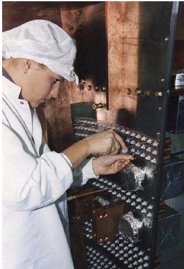
FIG. 3.51 – Photography of a petal sector during wiring. The operator blocked up the tapered half-cylinder in copper for an anode wire.
