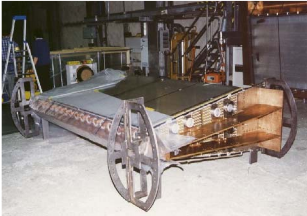
FIG. 3.89 – One sector in the LSM with its half-wheel system for rocking motion.
