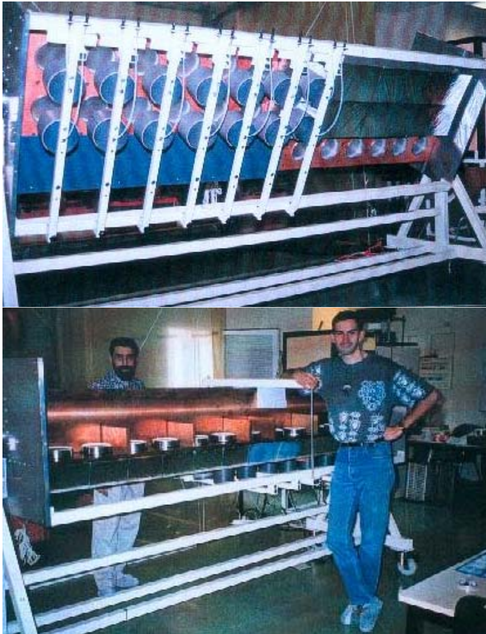
FIG. 3.37 – Scintillator mounting system on copper walls at CENBG.
