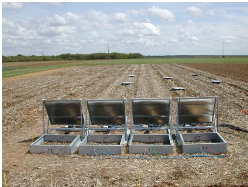
Illustration A: Gas chambers for the measurement of CO 2
