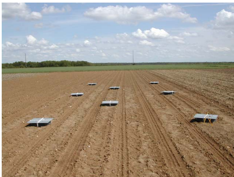
Illustration B: Gas chambers for the measurement of N 2 O
