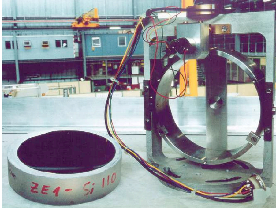
Figure 3.8 – Silicon crystal attached to the glass support and crystal holder. The holder has a step-by-step motor to adjust the crystal angle relative to the horizontal axis.
