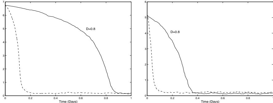
FIGURE 2.4.4. Substrate concentration taking initial conditions  $s_0 = 6.8\text{mg/L}$  (left) and  $s_0 = 5.1\text{mg/L}$  (right): Comparison between feedback control (dashed line) and fixed dilution (continuous line).
