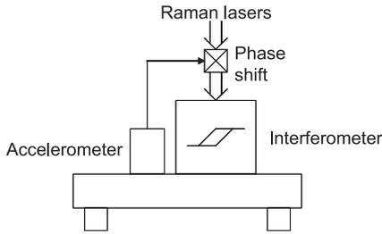
**Figure 8.** Principle of setup for acceleration compensation on the inertial sensor. The accelerometer signal is used to generate a correction signal on the Raman phase, which cancels the phase shift induced by vibrations.
