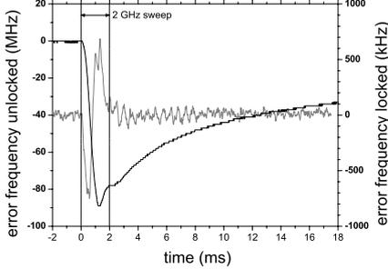
**Fig. 3** L2 frequency error during a 2 GHz sweep imposed in 2 ms. The black trace displays the frequency error when the servo loop is opened, and shows a sharp transient edge during the sweep, followed by an exponential like decay. The gray trace displays the frequency error when the servo loop is closed.
