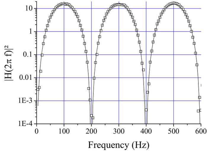
Fig. 5. The phase noise weighting function  $|H(2\pi f)|^2$  for  $T = 4.97$  ms and  $\tau_R = 20$   $\mu$ s, at low frequency. The theoretical calculation is displayed in solid line and the experimental results in squares. We clearly see the oscillating behavior of the weighting function and the experimental measurement are in good agreement with the theoretical calculation.
