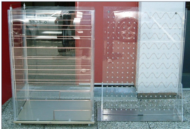
Figure 3.14: Comparison between double and sinusoidal MLA
