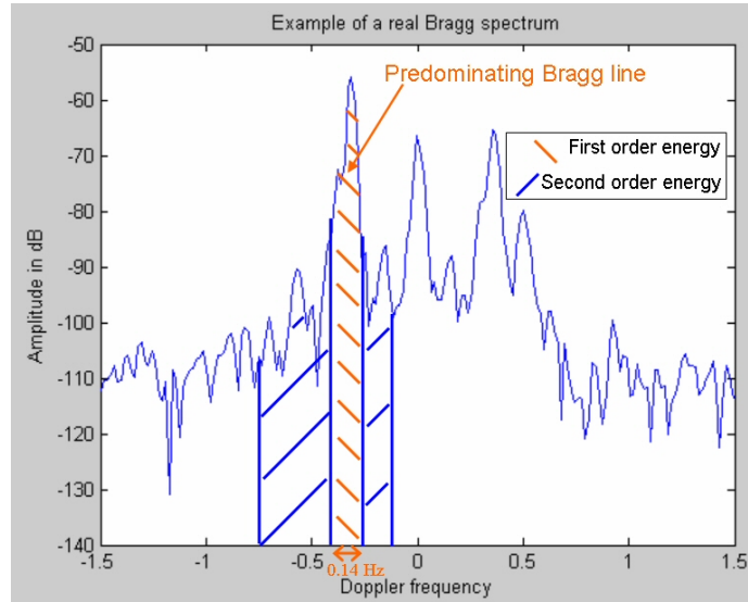
Figure 4.7: Repartition of the energy around the predominating Bragg line in a real sea spectrum
