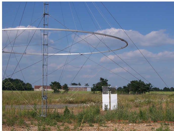
Figure 3.23: Comparison between the size of the compact HF antenna for low frequencies and a biconical antenna
