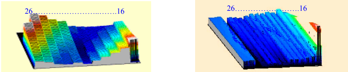
Figure 9 : Left: Profilometer view of all optical surfaces. Right: Profilometer view of back sides.
