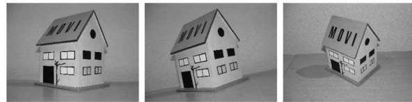
Fig. 3. Examples of singular and nonsingular configurations for calibration based on a parallelepiped with three right angles (the house's main body). Left: The parallelepiped's vertical edge is parallel to the camera's y -axis; this configuration is singular if the camera aspect ratio and principal point are not given (cf. cases B-3-0 and C-3-0 in Table 2). Middle: The parallelepiped's vertical edge is parallel to the image plane; this configuration is singular if the camera's principal point is not given (case B-3-0 in Table 2). Right: A rotation of the camera as shown here removes these singularities.
