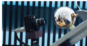
Figure 7: Catadioptric camera built from a Basler A201bc camera with a Fujinon 12.5 mm lens pointed at a roughly spherical mirror.
