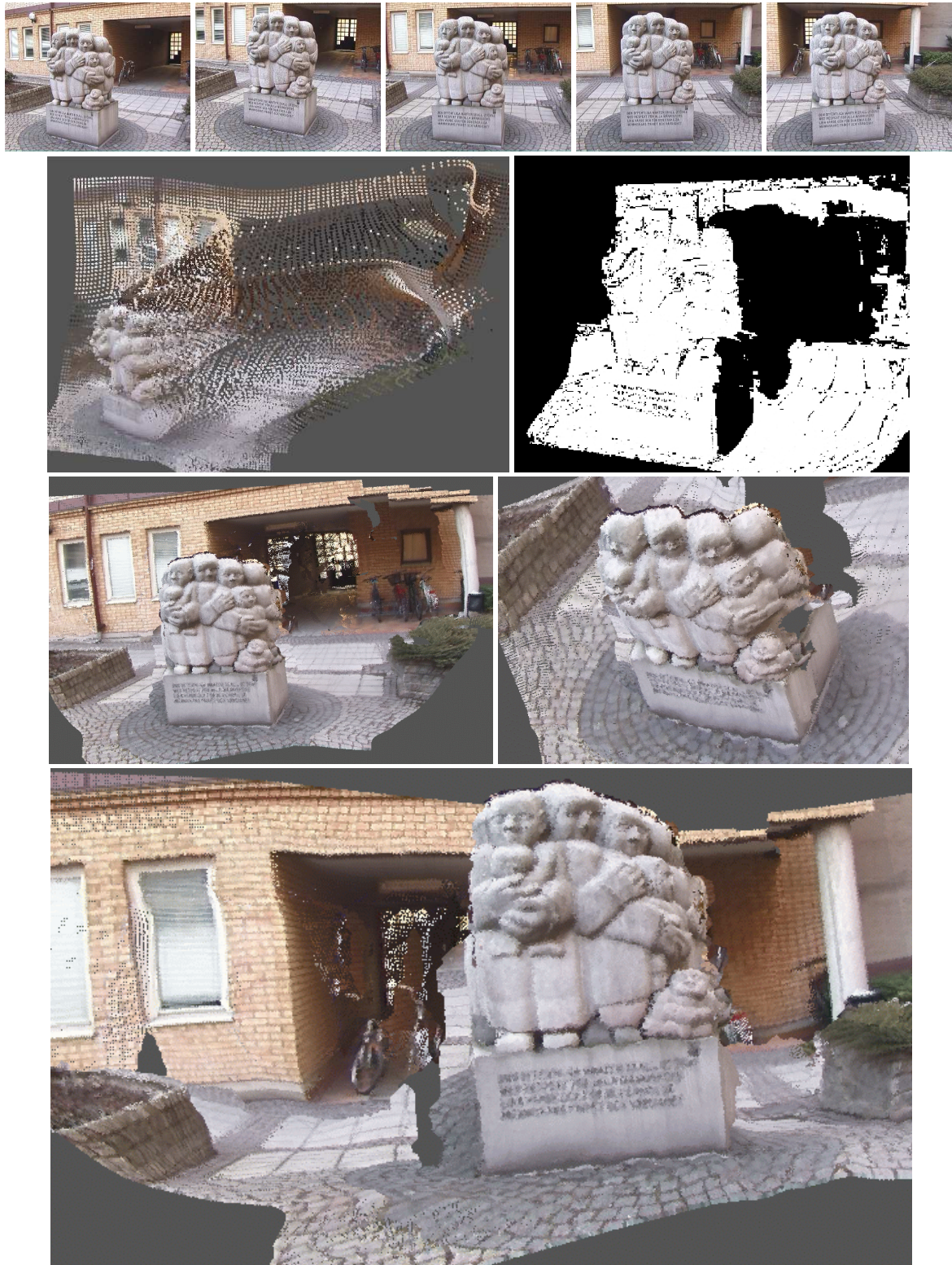
Figure 12.4: Top: five input images. Second row: initial model (obtained by “smoothing” the cloud of reconstructed interest points) and the estimated visibility map for the first input image relative to the third one (white means that the associated pixel of the first image is deemed likely to be visible in the third image). Bottom rows: texture-mapped 3D model. Parts of the background are only visible in one or two images and are necessarily badly reconstructed. The rest of the scene is quite well reconstructed though; especially, the large discontinuity between the statue and the background has been found completely.
