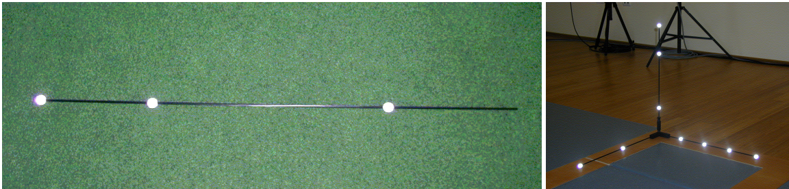
Figure 4.1: A calibration wand and a set of rigidly attached wands.
