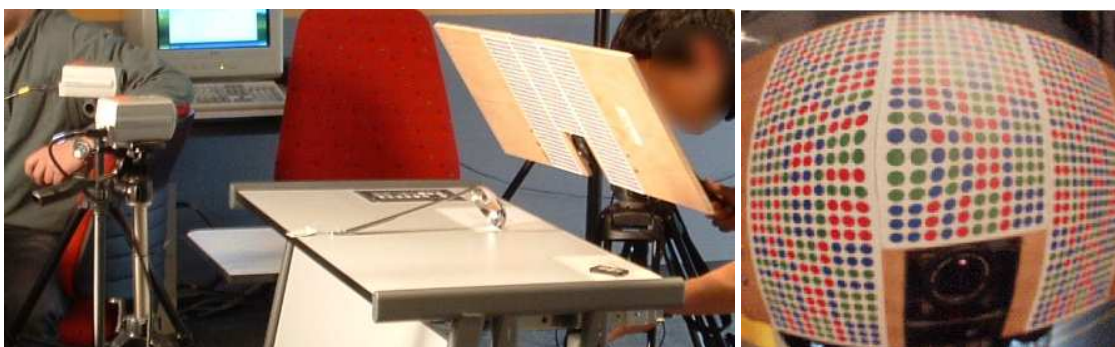
Figure 13.1: Left: experimental setup used in [19, 20]. The reference object is rigidly attached to the camera. The stereo system on the left is used to compute the displacement of the reference object, and thus of the camera. Right: a typical image of the reference object's reflection in the specular spoon.
