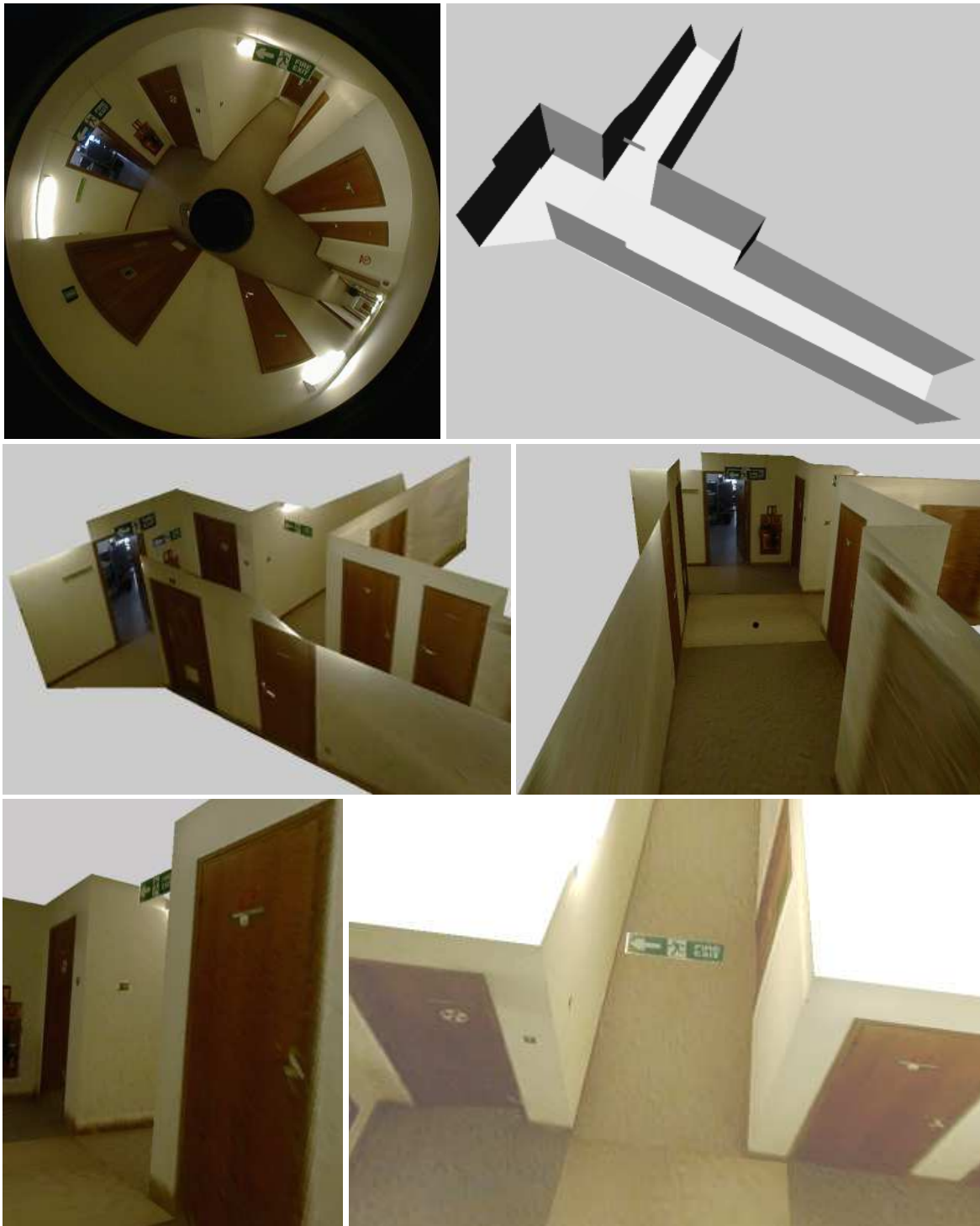
Figure 10.2: Results of 3D reconstruction from a single panoramic image, taken with a catadioptric camera. Top: input image and 3D model. Middle and bottom: renderings of the texture-mapped 3D model.
