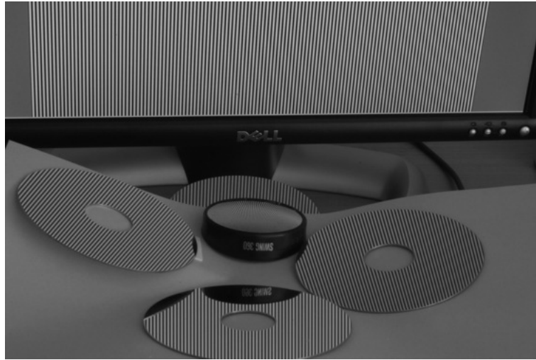
Figure 3.6: Experimental setup. This picture shows a view from our experimental setup. In the field of view of the camera, we see 4 planar mirrors, actually hard drive platters. At the top of the image, we have a direct view of the actual planar target. The curved mirror in the center of the image isn't used in this setup.
