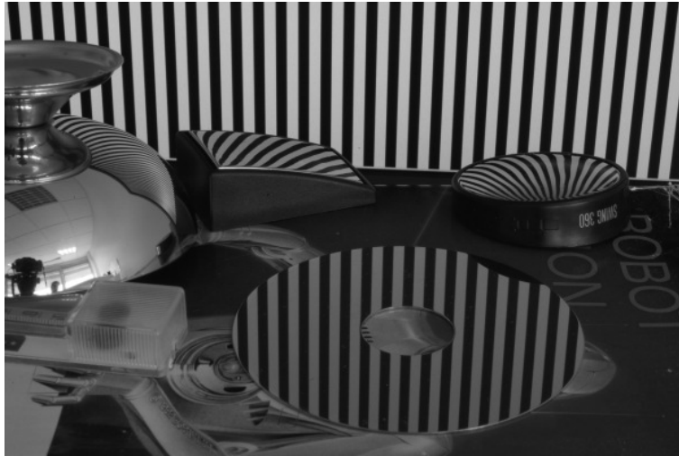
Figure 4.2: Direct view of a calibration pattern In this setup, the camera has a direct view of the calibration target (the LCD monitor) and of its reflection in the objects we wish to reconstruct.
