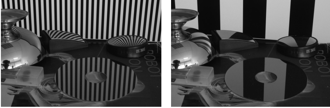
Figure 3.3: Experimental Setup. Two of the images used for the reconstruction. Notice the 3 curved mirrors (an ice-cream cup and two small wide-angle rear-view mirrors), the planar hard drive platter, and a direct view of the target plane (the LCD panel), in the upper part of the image. The pattern displayed on the LCD panel corresponds to the structured light approach presented in appendix A.
