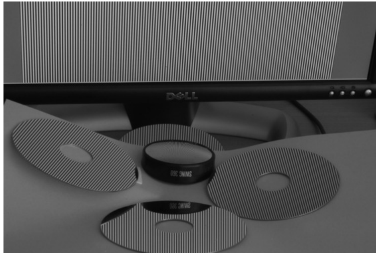
Figure 4.6: Experimental setup This picture shows a view from our experimental setup. In the field of view of the camera, we see 4 planar mirrors, actually hard drive platters. At the top of the image, we have a direct view of the actual planar target. The curved mirror in the center of the image isn't used in this setup.
