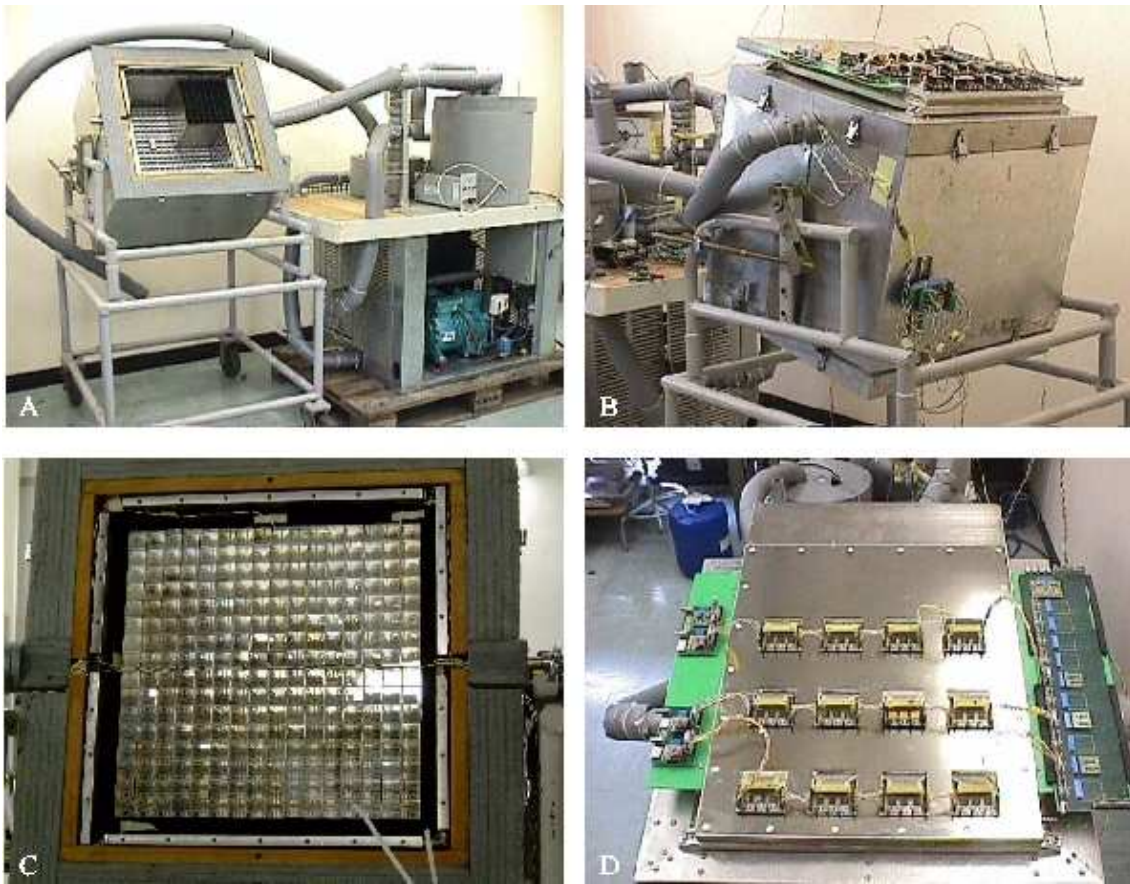
Figure 4.2: The 256 crystal PHOS prototype. A: Detector and cooling system. B: Closed detector with CPV on top. C: Crystal matrix. D: Close-up of the CPV.
