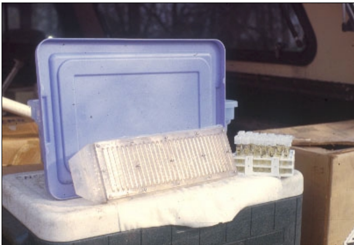
Figure 3-1: Illustration of a sediment porewater sampler (lying horizontally) after collection on the field. Water samples from each slot were stored in glass vials and put on ice in the field before storage in the laboratory at 4°C (right of the sampler)
