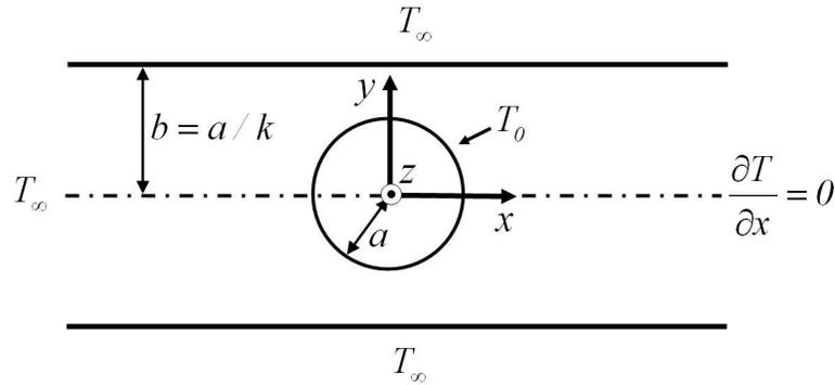
FIG. 2.1 – Conditions aux limites de type Dirichlet
