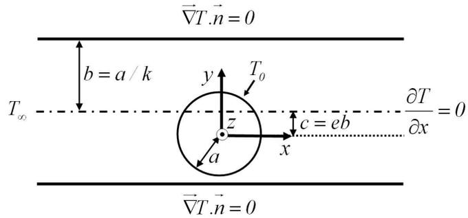
FIG. 3.10 – Conditions aux limite de type Neumann
