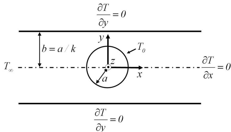
FIG. 2.10 – Conditions aux limites de type Neumann
