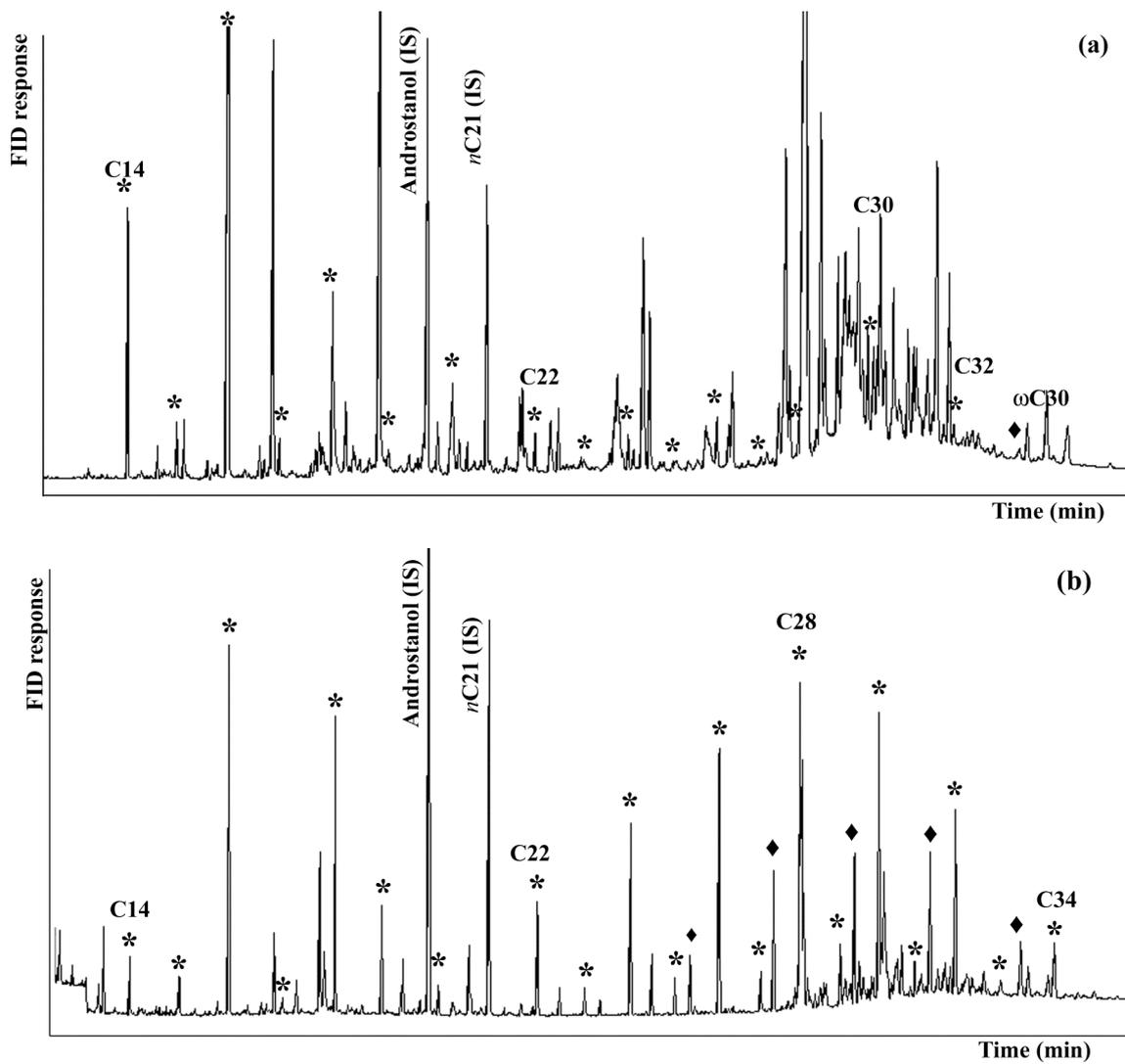
Fig. 2: Gas chromatograms of the F4 fraction of the extracts of the material from the 400 m Pelagic trap (a) and from the 30 m Turbidite trap (b), showing *n*-alcohols from C<sub>14</sub> to C<sub>34</sub> (\*) and ω-hydroxy acid from C<sub>22</sub> to C<sub>30</sub> (◆) (IS= internal standard).
