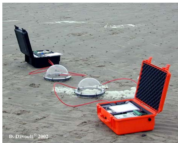
Fig. 2 Example of simultaneous measurement of benthic metabolism on bare sediment (middle ground) and a small Phaeocystis foam deposit (foreground)
