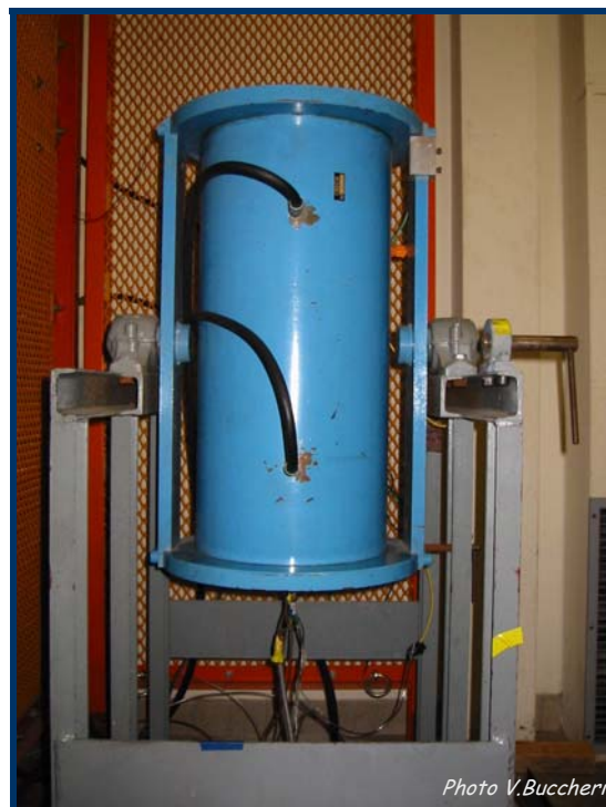
fig. 3.2: front vision of Internally Heated Pressure Vessel working vertically (Gros Bleu), equipped with a fast quench device. The two black rubber pipes ensure water circulation for the cooling of the furnace. Thermocouples exit wires are visible in the lower part of the vessel. CNRS-ISTO, Orléans- France.
