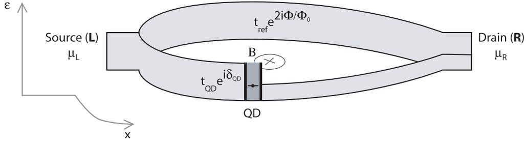
Figure 4.14: Sketch of an Aharonov-Bohm interferometer ring. The electron from the source ( $\mu_L$ ) can reach the drain ( $\mu_R$ ) through either the upper (reference) or lower arm which the quantum dot is embedded in.
