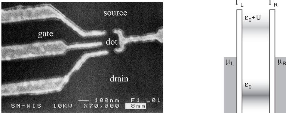
Figure 1.4: Left: Scanning electron microscope image of a typical quantum dot (top view). The black regions indicate the 2DEG, gray regions indicate the metal gates [29]. Right: Schematic representation of quantum dot structure.
