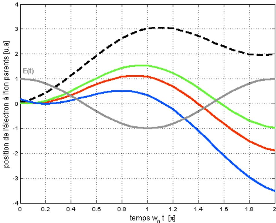
FIGURE 2.5: TRAJECTOIRES POSSIBLES D'UN ÉLECTRON LIBRE DANS LE CHAMP LASER EN FONCTION DE SES INSTANTS DE NAISSANCE (PHASE DE NAISSANCE  $\omega_0 t_i$ ) DANS LE CONTINUUM : TRAJECTOIRES (POINTILLE) OU L'ÉLECTRON NE RETOURNE PAS A L'ION PARENT (SUPPOSE IMMOBILE EN POSITION 0), TRAJECTOIRE DE LA COUPURE (ROUGE), TRAJECTOIRE COURTE DU PLATEAU (BLEU) ET TRAJECTOIRE LONGUE DU PLATEAU (VERT).
