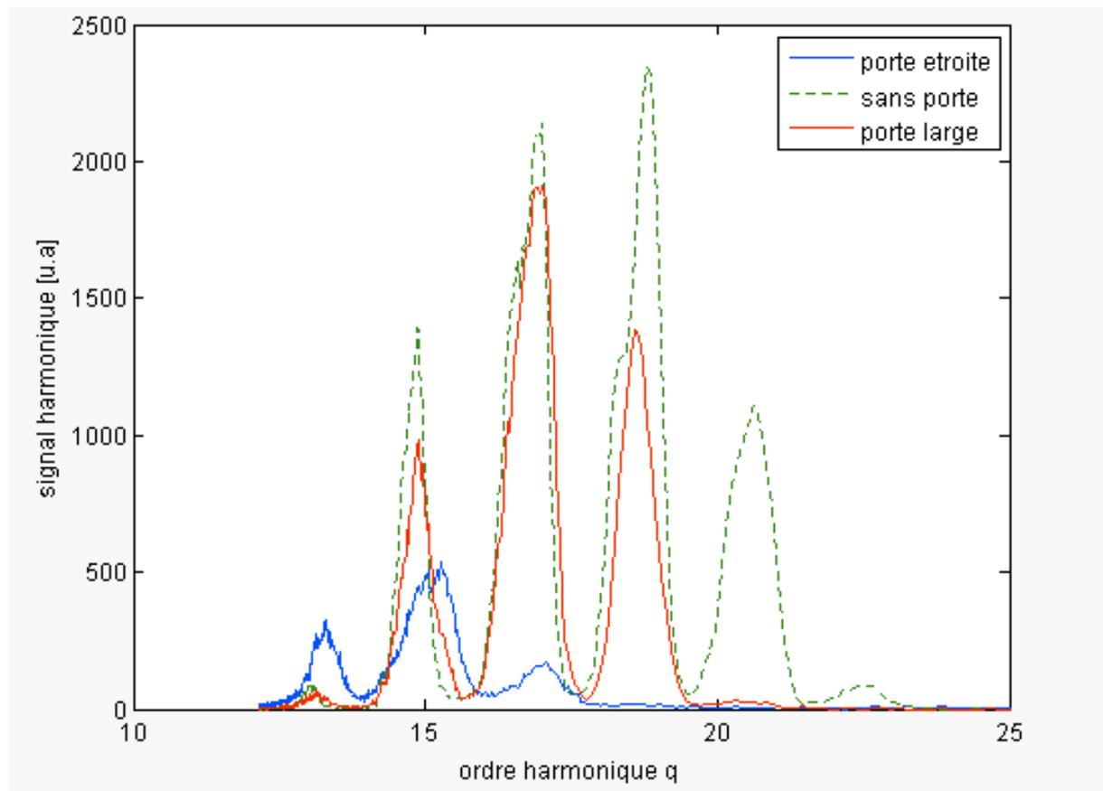
FIGURE 2.2 : SPECTRE HARMONIQUE GÉNÉRÉ DANS L'ARGON PAR UNE IMPULSION LASER DE 10 fs ET UNE PORTE D'ELLIPTICITE ( $\delta\tau=10$  fs) EN CONFIGURATION SANS PORTE, PORTE LARGE ET PORTE ÉTROITE.
