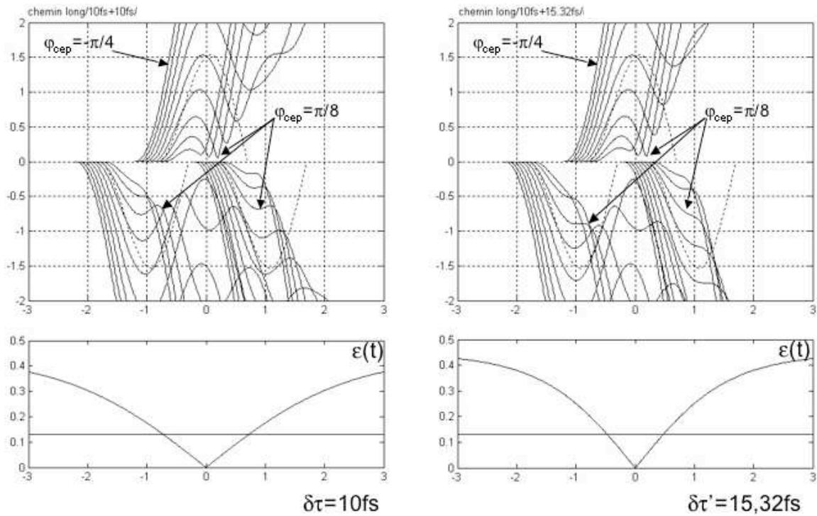
FIGURE 1.13: TRAJECTOIRES ÉLECTRONIQUES CORRESPONDANT AU CHEMIN LONG, EN FONCTION DE LA PHASE ABSOLUE LASER, INDUITES PAR UNE IMPULSION LASER DE 10 fs ET UNE PORTE D'ELLIPTICITÉ POUR DES DÉLAIS  $\delta\tau=10$  fs (GAUCHE) ET  $\delta\tau'=15,32$  fs (DROITE).
