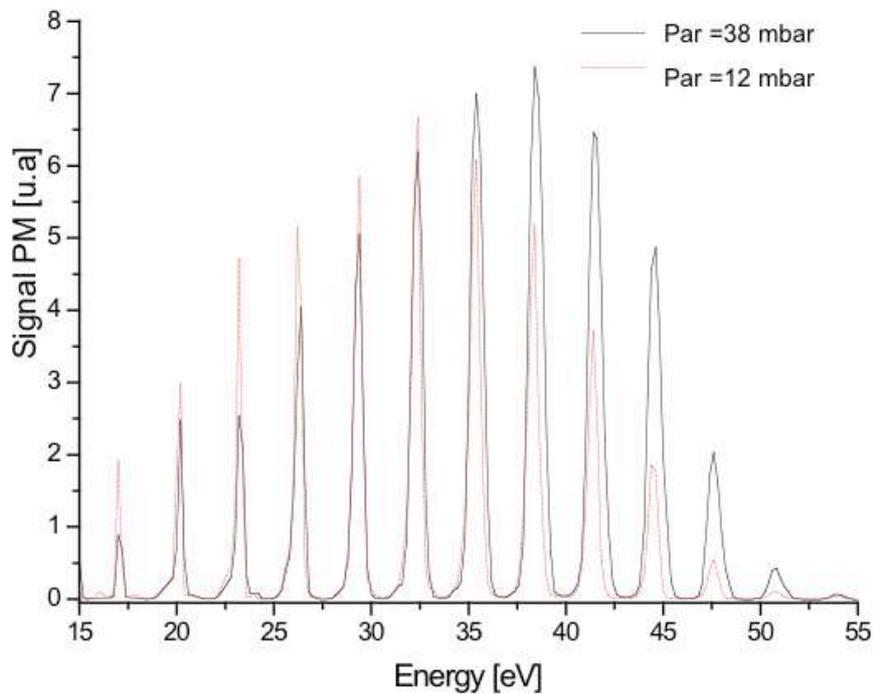
FIGURE 2.14: SPECTRE HARMONIQUE OBTENU DANS L'ARGON POUR DEUX PRESSIONS : 12 MBAR (POINTILLÉ) OPTIMISE LES HARMONIQUES DU PLATEAU ET 38 MBAR (CONTINU) OPTIMISE LES HARMONIQUES DE LA COUPURE.
