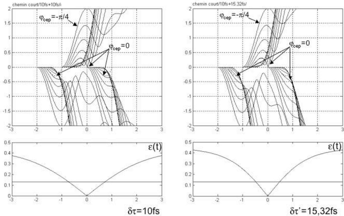
FIGURE 1.15 : TRAJECTOIRES ÉLECTRONIQUES CORRESPONDANT AU CHEMIN COURT, EN FONCTION DE LA PHASE ABSOLUE LASER, INDUITES PAR UNE IMPULSION LASER DE 10 fs ET UNE PORTE D'ELLIPTICITÉ POUR DES DÉLAIS  $\delta\tau=10$  fs (GAUCHE) ET  $\delta\tau'=15,32$  fs (DROITE).
