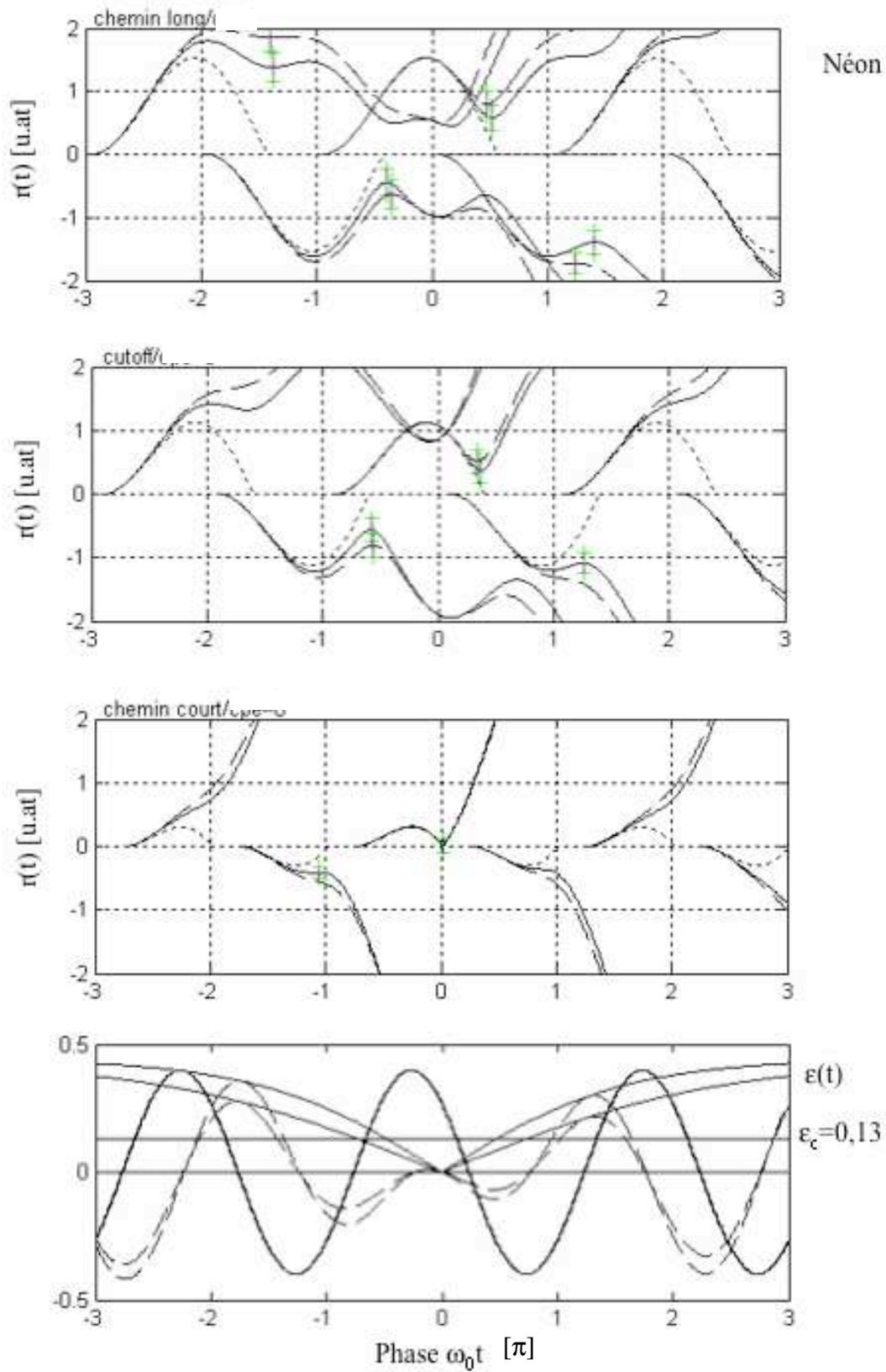
FIGURE 1.12: TRAJECTOIRES ÉLECTRONIQUES CALCULEES POUR LE CHEMIN LONG, LA COUPURE ET LE CHEMIN COURT, GENEREES PAR UNE IMPULSION LASER DE 10 fs ET UNE PORTE D'ELLIPTICITE DE DÉLAIS  $\delta\tau=10$  fs (CONTINU) ET  $\delta\tau'=15,32$  fs (TRAIT).
