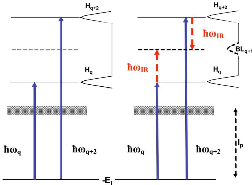
FIGURE 2.4 : IONISATION AU-DESSUS DU SEUIL PAR DES PHOTONS HARMONIQUES  $\hbar\omega_q$  ET  $\hbar\omega_{q+2}$  (A) ET HABILLAGE PAR ABSORPTION OU EMISSION D'UN PHOTON IR  $\hbar\omega_{IR}$  (B) CONDUISANT À L'APPARITION D'UNE BANDE LATÉRALE INTER-HARMONIQUE  $BL_{q+1}$ .
