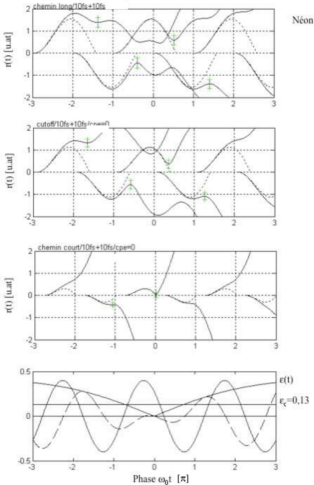
FIGURE 1.11: TRAJECTOIRES ÉLECTRONIQUES CALCULEES POUR LE CHEMIN LONG, LA COUPURE ET LE CHEMIN COURT, GENERE PAR UNE IMPULSION LASER DE 10 fs ET UNE PORTE D'ELLIPTICITE DE DELAI  $\delta\tau=10$  fs EN CONFIGURATION PORTE ETROITE (CONTINU) ET PORTE LARGE (POINTILLE). LA DISPERSION DU PAQUET D'ONDE ELECTRONIQUE (BARRES D'EREURS) ET ICI PRIS EN COMPTE.
