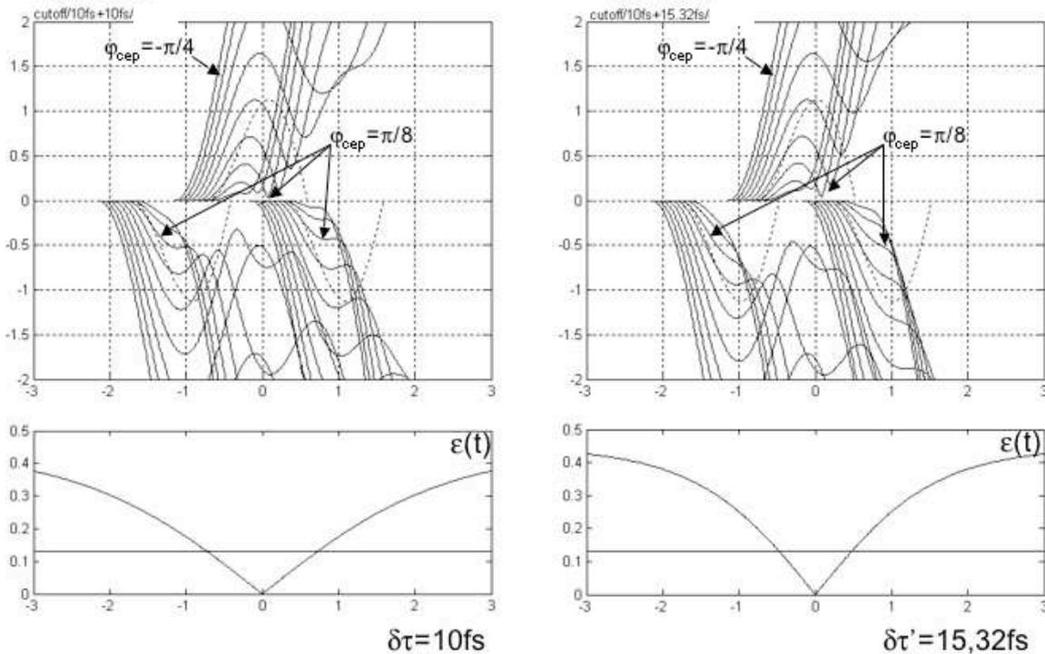
FIGURE 1.14 : TRAJECTOIRES ÉLECTRONIQUES CORRESPONDANT A LA COUPURE, EN FONCTION DE LA PHASE ABSOLUE LASER, INDUITES PAR UNE IMPULSION LASER DE 10 FS ET UNE PORTE D'ELLIPTICITÉ POUR DES DÉLAIS  $\delta\tau=10$  fs (GAUCHE) ET  $\delta\tau'=15,32$  fs (DROITE).
