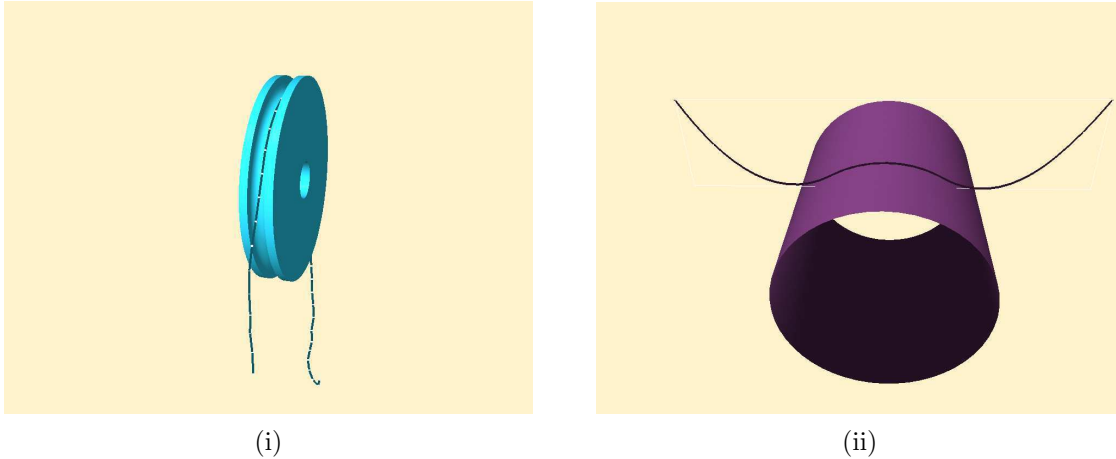
Fig. 5.9: Snapshots of simulation using QP-Collide. A stiff cable (i) falling off a pulley and (ii) suspended (fixed at the end points) over a cylinder.
