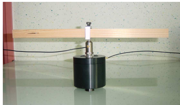
Figure I- 8 : Dispositif expérimental “fixed-free flexural vibration method”
