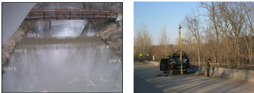
(a) LSPIV processing area within 6 GRPs (b) Deployment of MLSPIV
