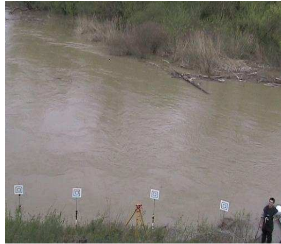
Figure 4. LS-PIV picture during 2005, April 8 th flood The left-bank 4 Ground Reference Points installed at the same elevation
