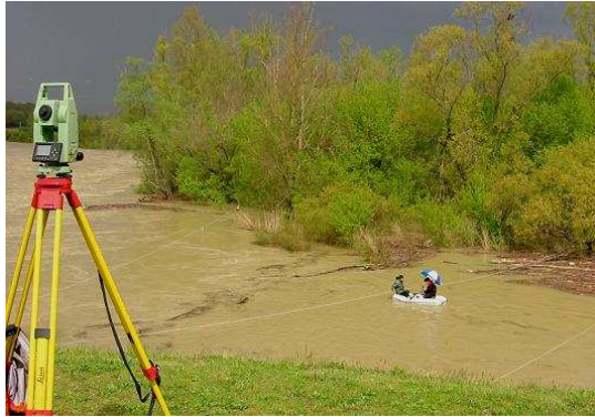
Figure 3. ADcp deployment during 2005, April 25 th flood The Ain river is flowing from the top left corner; transects A, B, C are delimited by white tight ropes
