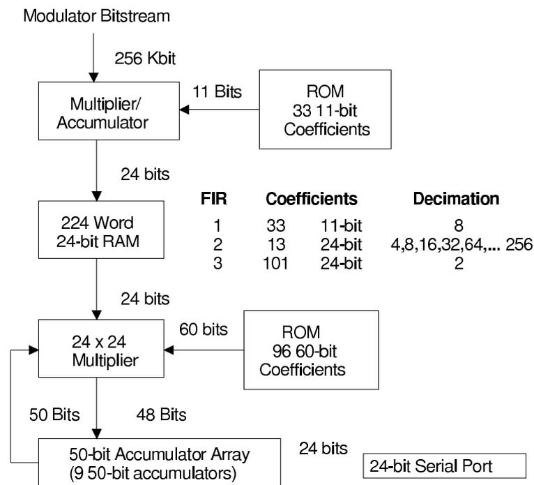
Figure 1. Digital Filter Block Diagram
