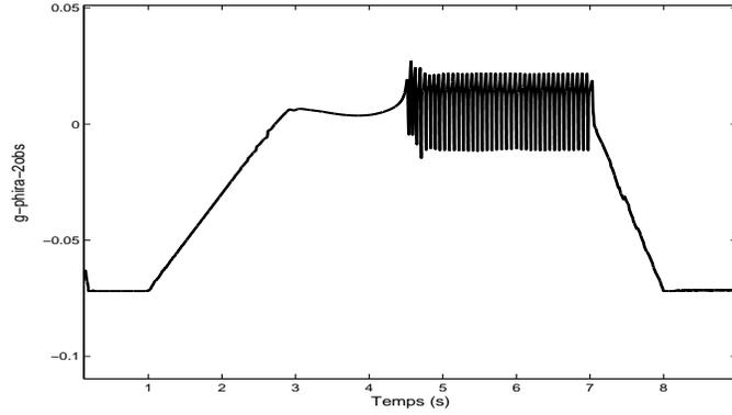
FIG. B.12: Gain de flux rotorique  $\phi_{r\alpha}$ .
