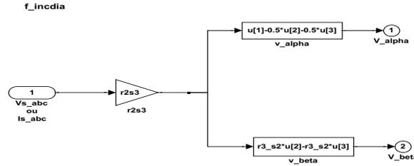
FIG. C.3: vs\_abc2vs\_alpha, beta ou Is\_abc2Is\_alpha, beta.
