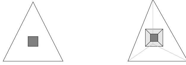
Figure 3.8: An example of the external hypertriangles used to avoid open Voronoi regions in 2D (left) and 3D (right). The dark gray area identifies the input space
