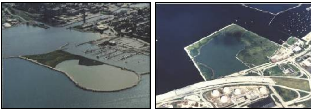
Photo 1-3: stockages confinés aux USA : Milwaukee et Bolles (Source: http://www.lrd.usace.army.mil )
