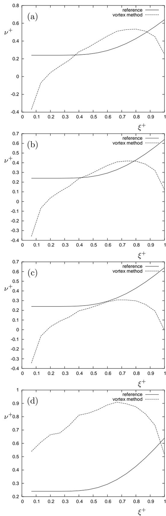
FIG. B.4 – Spectral numerical viscosity of the vortex method with a combination of  $M'_4$ ,  $\Lambda_3$  and  $M_4$  with respective coefficients (a)  $c = (0.5, 0.5, 0.0)$ , (b)  $c = (0.6, 0.4, 0.0)$ , (c)  $c = (0.7, 0.3, 0.0)$ , and (d)  $c = (0.599, 0.4, 0.001)$ .
