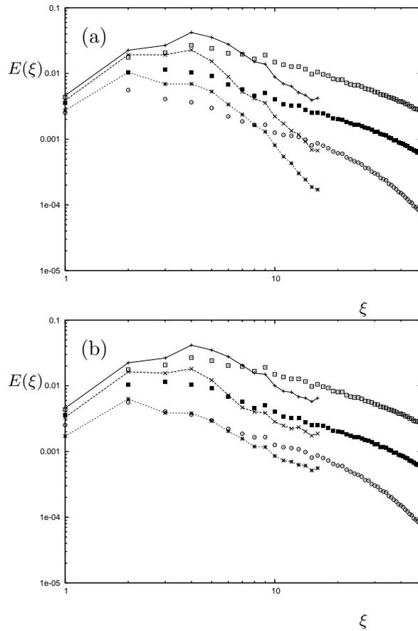
FIG. B.7 – Instantaneous 3D energy spectra for LES with the VIC method of the Comte-Bellot – Corrsin experiment, LES with  $32^3$  cells/particles,  $dt = 0.03$ . (a) Remeshing performed with a combination of  $M'_4$  and  $\Lambda_3$  (0.6, 0.4, 0.0). (b) Remeshing performed with a combination of  $M'_4$ . Crosses represent DNS data of A. Wray [86]. (+  $t' = 42$ ,  $\times$   $t' = 98$  and  $*$   $t' = 171$ ), symbols denote the present LES.
