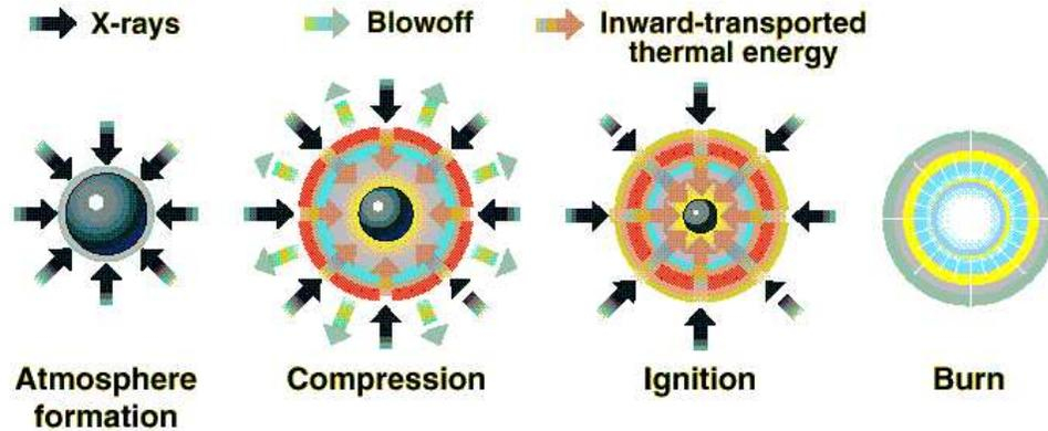
The X-rays rapidly (1) heat the capsule, (2) causing its surface to fly outward. This outward force causes an opposing inward force that compresses the fuel inside the capsule. When the compression reaches the center, temperatures increase to 100,000,000 °C, (3) igniting the fusion fuel and (4) producing a thermonuclear burn that yields many times the energy input (energy gain).
