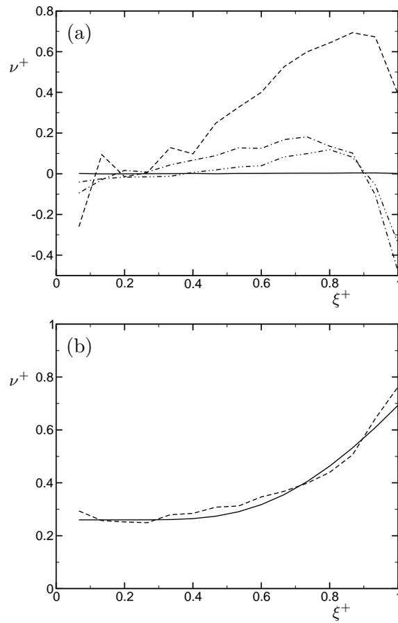
FIG. B.1 – Spectral numerical viscosity of (a) — de-aliased spectral method, ·-·-·- 2nd-order central FD, -·-·-· 4th-order central FD, - - - - 2nd-order central FD with staggered grid. (b) — EDQNM theory [?], - - - - ALDM with optimized parameters [41].
