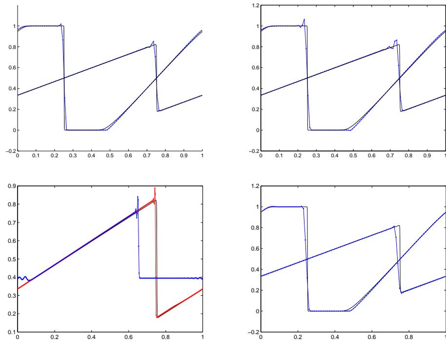
FIG. C.1 – Comparison of Lax-Wendroff (LW) and particle schemes. Top row : LW (left) and particle (right) schemes with  $h = 0.01$ , artificial viscosity coefficient 0.2 and  $\mu = 0.84$ . Bottom left : LW (blue curve) and particle (red curve) schemes without artificial viscosity at  $t = 1.5$  and  $h = 0.0025$  . Bottom right, particle method with adaptive time-step and  $h = 0.01$ .
