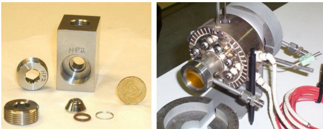
Figure 3.6: Cunsolo cell (left panel) and the HP cell used for the study of supercritical water and ammonia (right panel).
