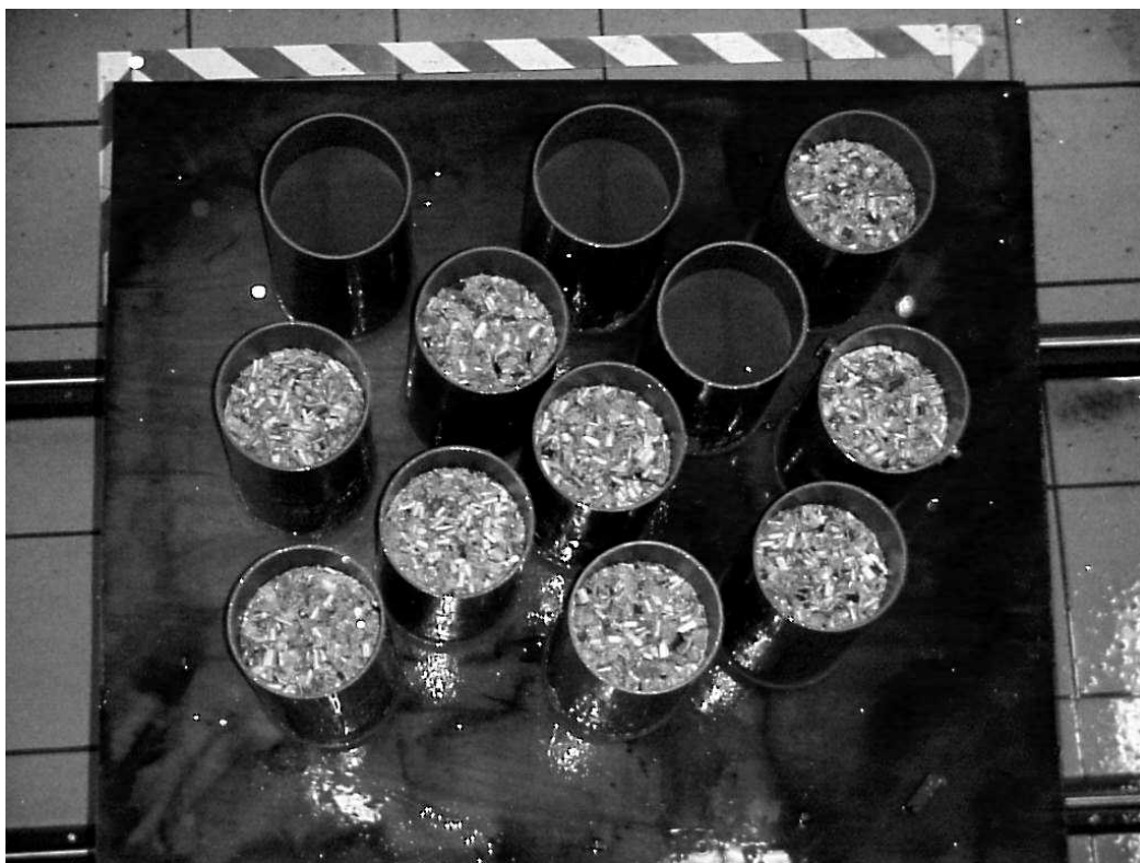
Picture A.3 View of the soil columns (30 cm length and diameter of 15 cm) placed under the rain simulator, with residues left at the soil surface or incorporated in the upper 10 cm of the soil
